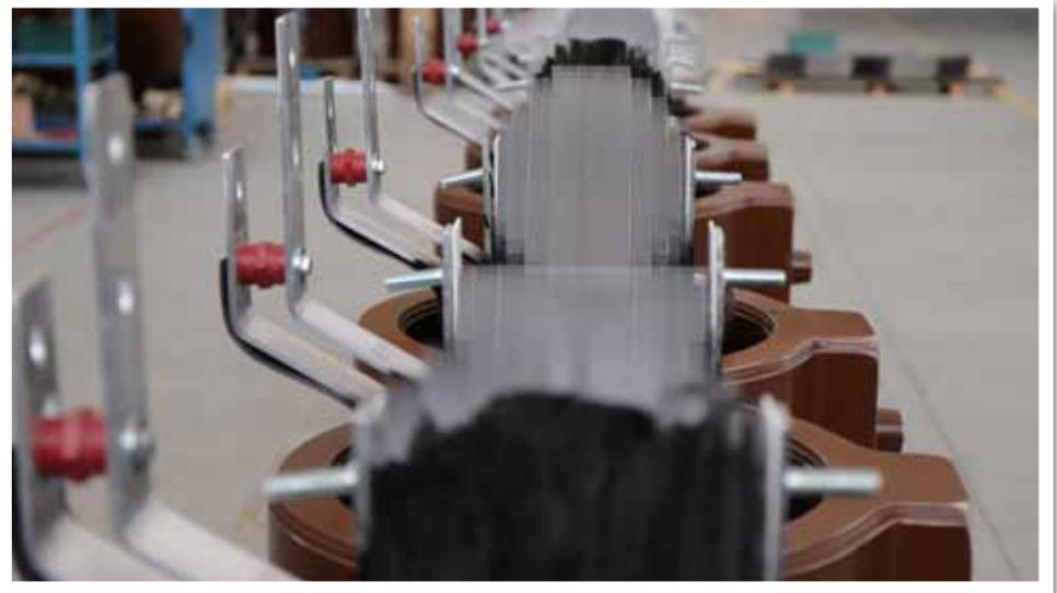
Fig. 5 - View of the lamination of the core.
