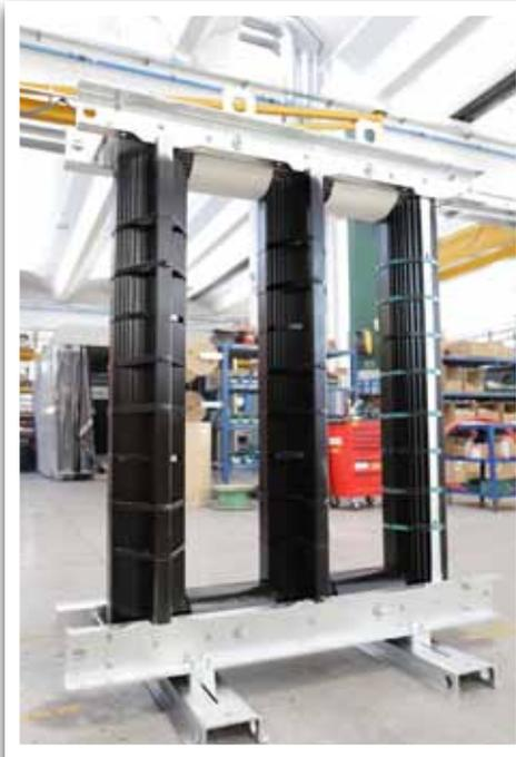
*Fig. 10 - Magnetic core.*
