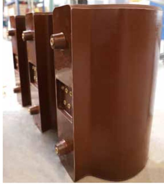
Fig. 7 - Typical high Voltage Winding.
