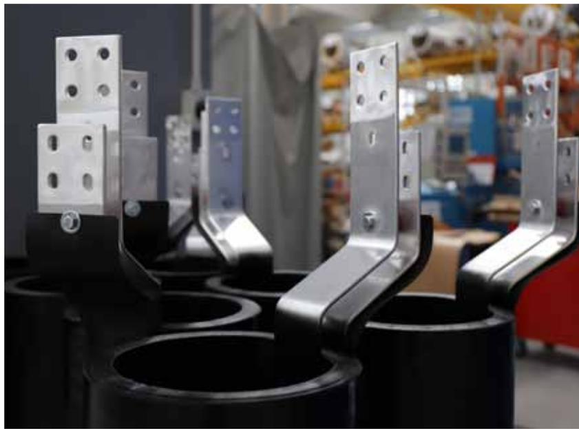
Fig. 6 - Typical cast resin low voltage winding.
