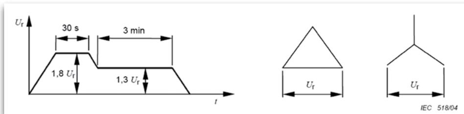
Fig. 19 - Voltage application for routine partial discharge test.
