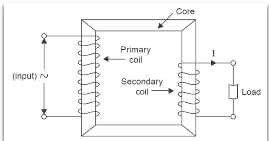
Fig. 1 - Primary coil is energized, secondary coil is loaded.
