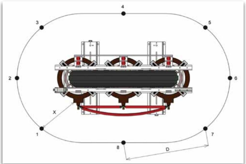
Fig. 16 - Microphone positions for point-by-point measurement.
