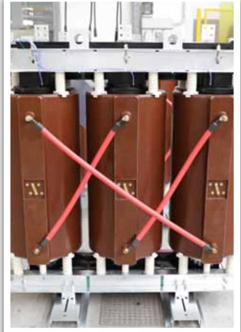
*Fig. 12 - Completed cast resin transformer ready for test.*
