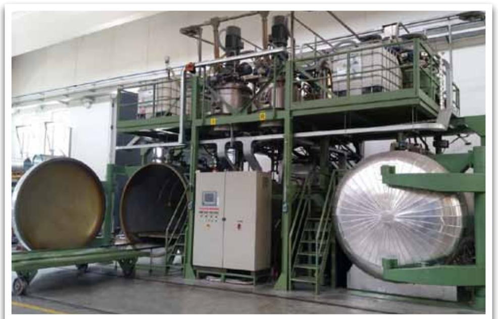
Fig. 9 - Autoclave for high voltage coils.
