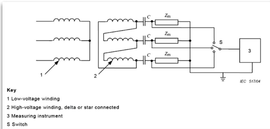
Fig. 18 - Basic measuring circuit for the partial discharge test for a three-phase transformer
