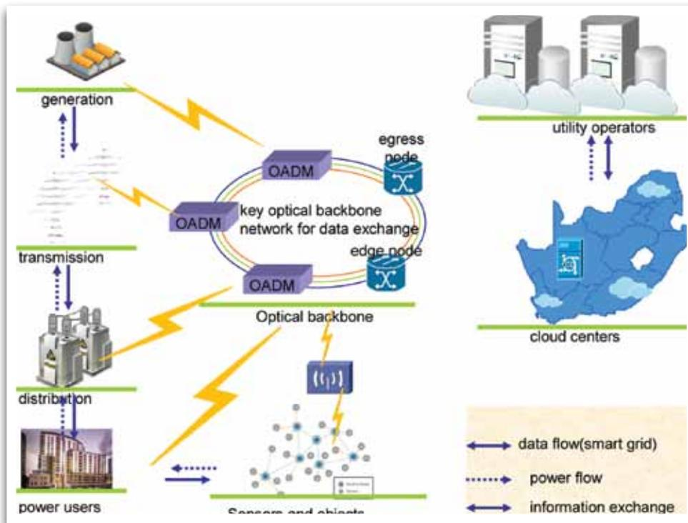
Figure 1: Smart Grid and support Network infrastructure
