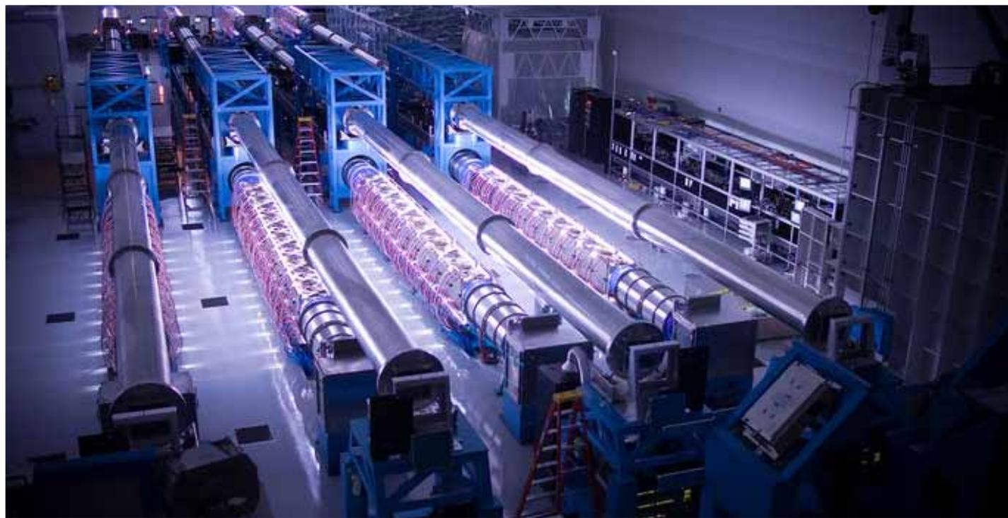
*Amplifiers for the University of Rochester's OMEGA-EP, lit up by flash lamps, could drive a U.S. high-power laser.*
