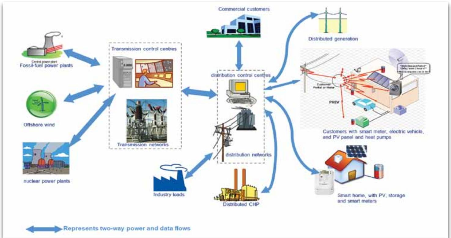
Figure 2: Smart Grid Example (Merz and McLellan)
