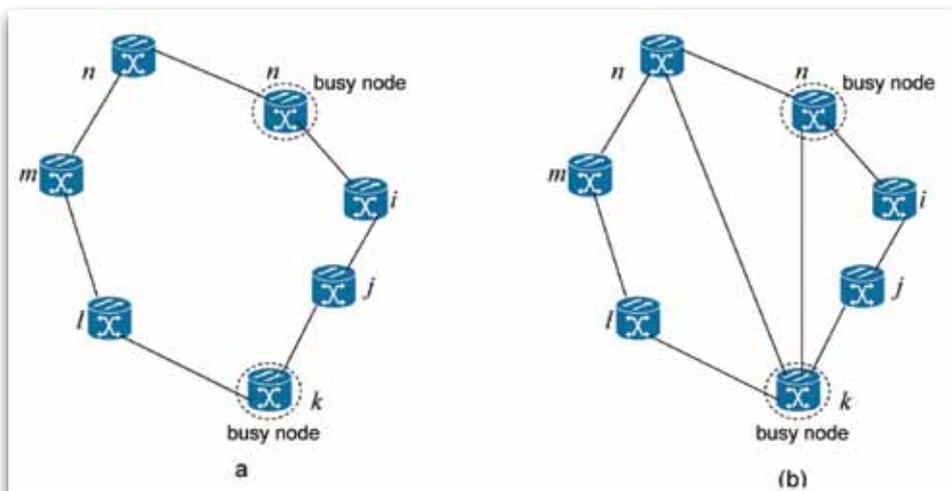
Figure 2. Networking topologies: (a) ring and (b) mesh [6].
