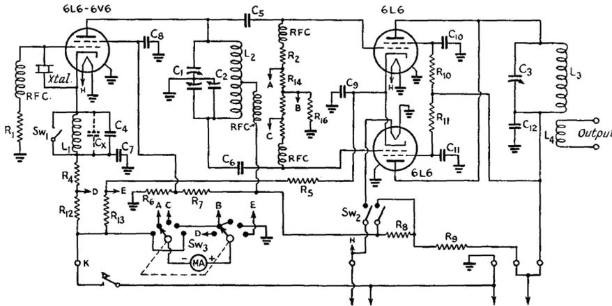
Fig 6: A proposed circuit diagram of the CW exciter of the transmitter.
