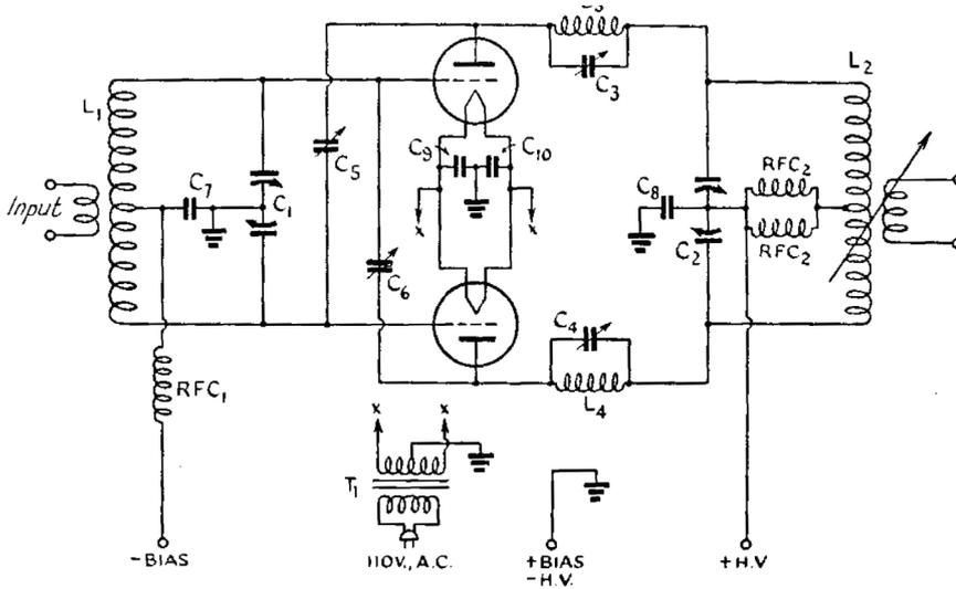
Fig 5: A suggested circuit diagram of the power amplifier of FELIX's transmitter.
