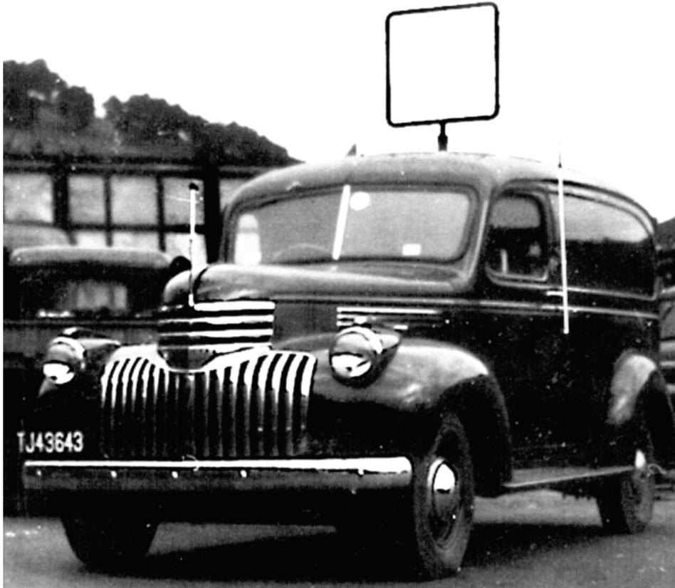
Fig 4: A Price-Milne Organisation mobile direction-finding vehicle with its loop antenna.
