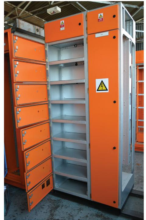
*A semi-assembled motor control centre at Shaw Controls showing the aluzinc framework.*
