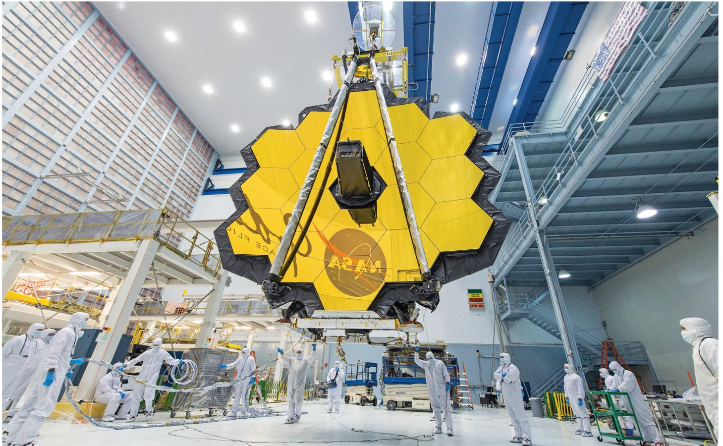
*The James Webb Space Telescope would be the most complex imaging hardware that NASA has attempted to put into space. It features a large mirror that will be formed by multiple individual segments moving into place and protected by a sunshield that would also unfold after launch.*
