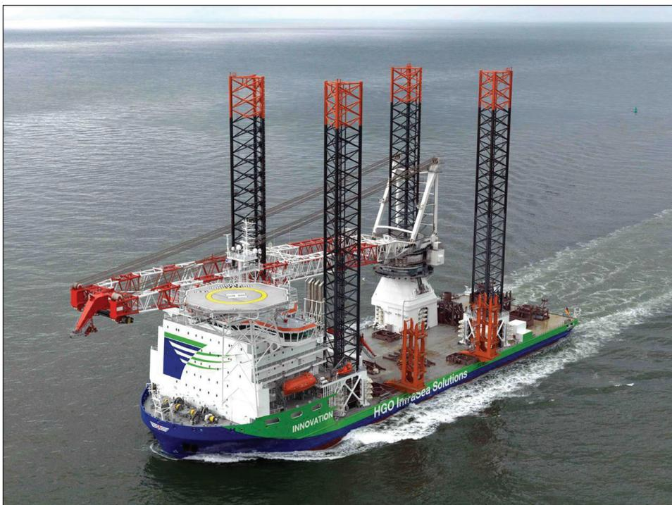
*Ship Innovation – has a load capacity of 8,000 tons and can install in waters up to a 65 meter depth.*
