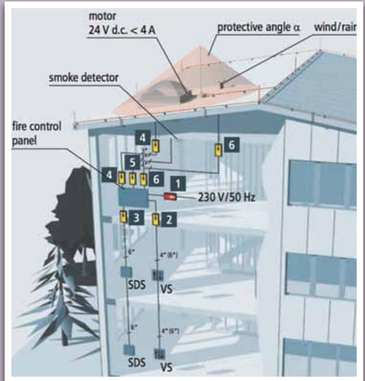
Figure 1: Domelight located in the protected volume of an air-termination rod on a non-metal roof of a structure with external lightning protection system.
