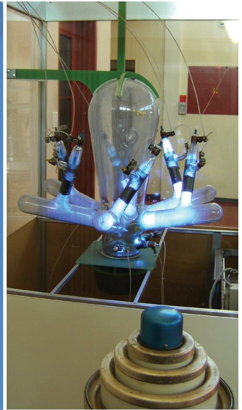
Three-phase mercury arc rectifier
