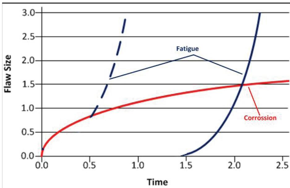
Figure 4: Example of a possible built-in model showing how corrosion strongly influences damage due to mechanical effects in structures. [source: Lunar Inc.]
