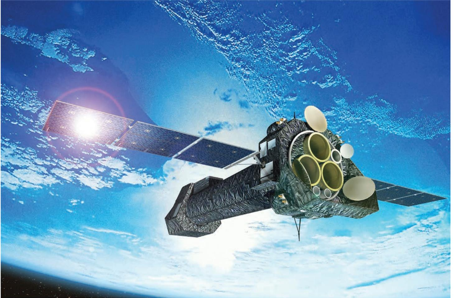
*An assembly of 51 mirrors, carefully sized, formed and nested one inside another, makes XMM-Newton the most sensitive X-ray telescope ever built. ESA's XMM-Newton derives its name from its X-ray multi-mirror design and honours Sir Isaac Newton. This unique X-ray observatory was launched by Ariane 5 from the European spaceport in French Guiana on 10 December 1999.*
