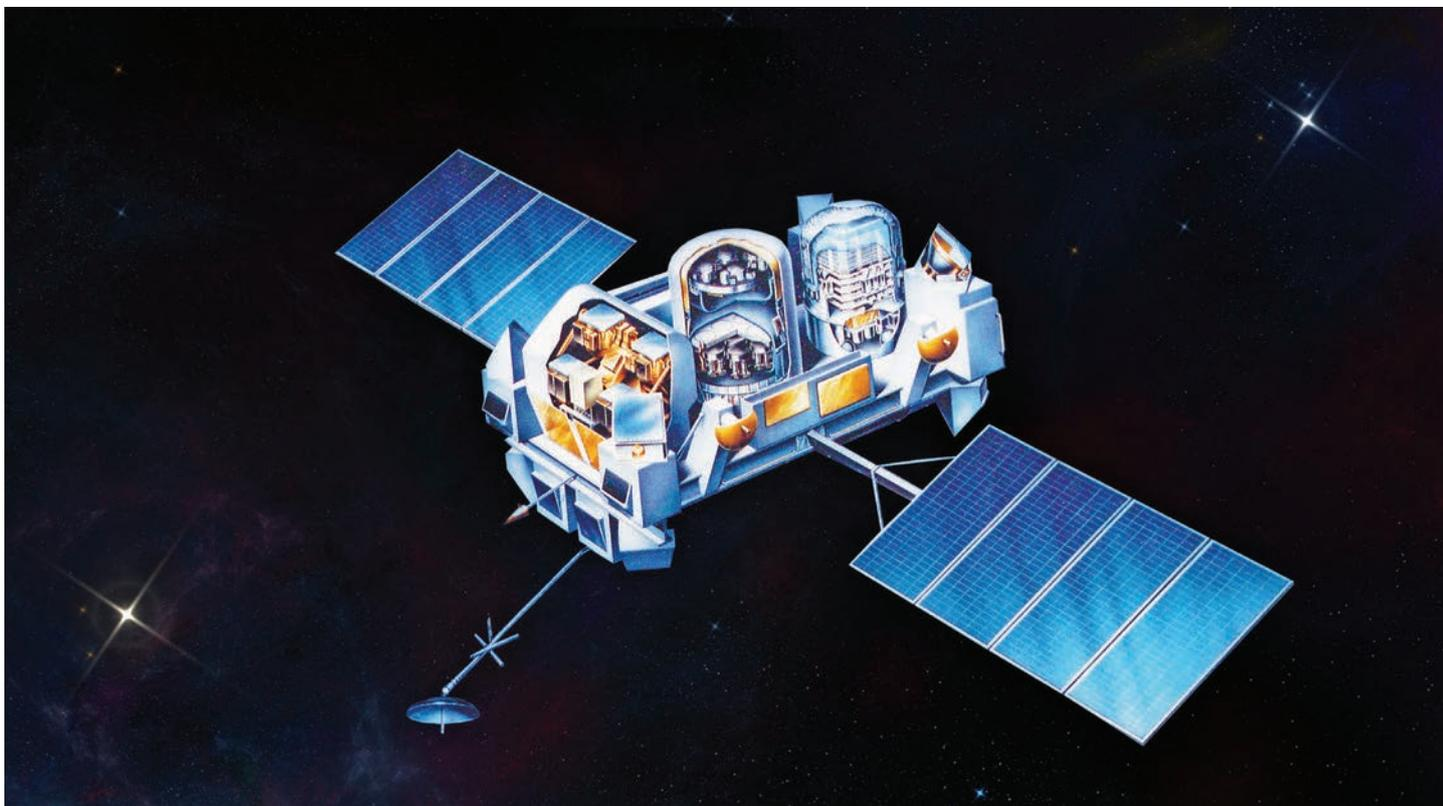
*This illustration of the Compton Gamma Ray Observatory shows the locations of its four instruments, the Burst And Transient Source Experiment (BATSE), the Oriented Scintillation Spectrometer Experiment (OSSE), the Imaging Compton Telescope (COMPTEL), and the Energetic Gamma Ray Experiment Telescope (EGRET).*
