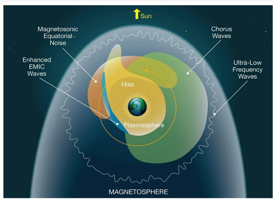
*Different types of plasma waves triggered by various mechanisms, occupy different regions of space around Earth.*
