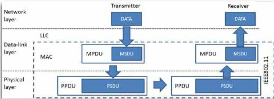
Figure 4: Simplified view of OSI model and packet encapsulation.
