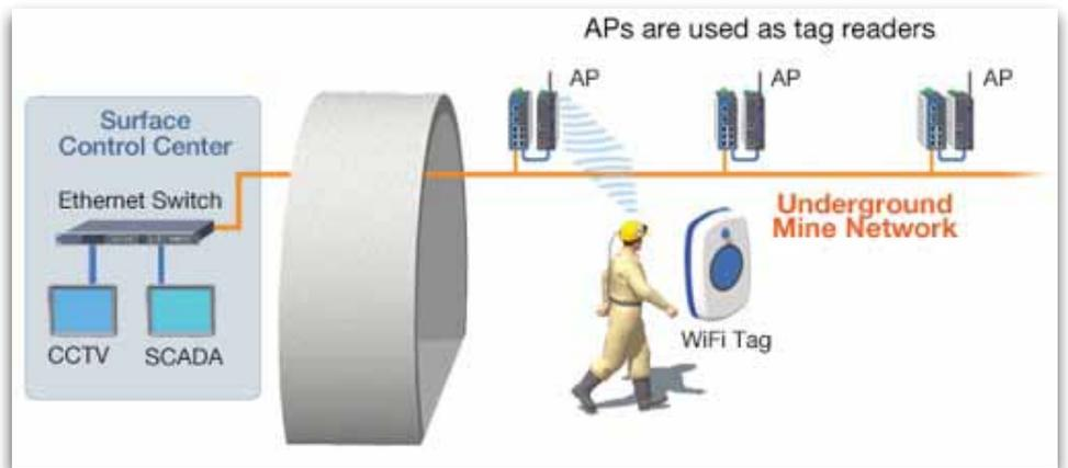
Figure 8: Example of real-time location tracking [source: 9]
