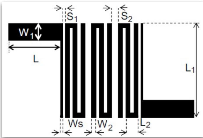
Figure 1: Two-dimensional design of three-polar band-pass filter
