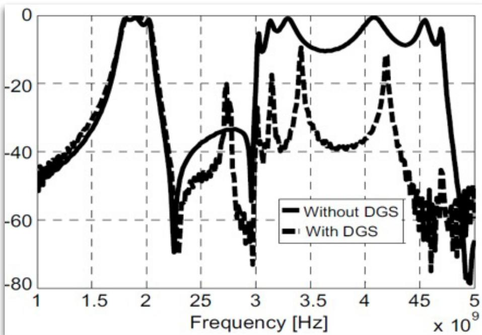
Figure 8: Compare S21 response of filter with DGS plate and non-DGS plate
