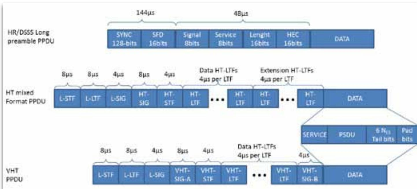
Figure 6: Example physical layer frame formats with 802.11b, n and ac. [source: EKAHU]
