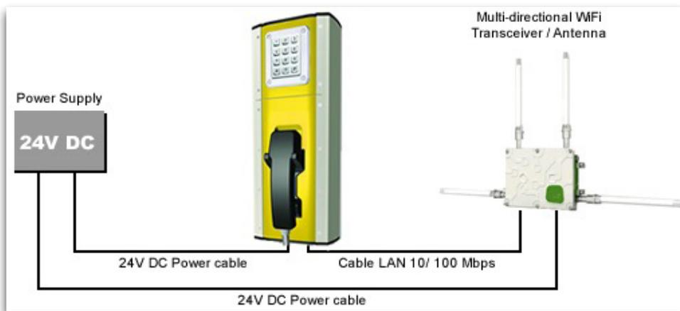
Figure 2: A Wireless Emergency Telephone system [source: [www.norphonic.com](http://www.norphonic.com)]
