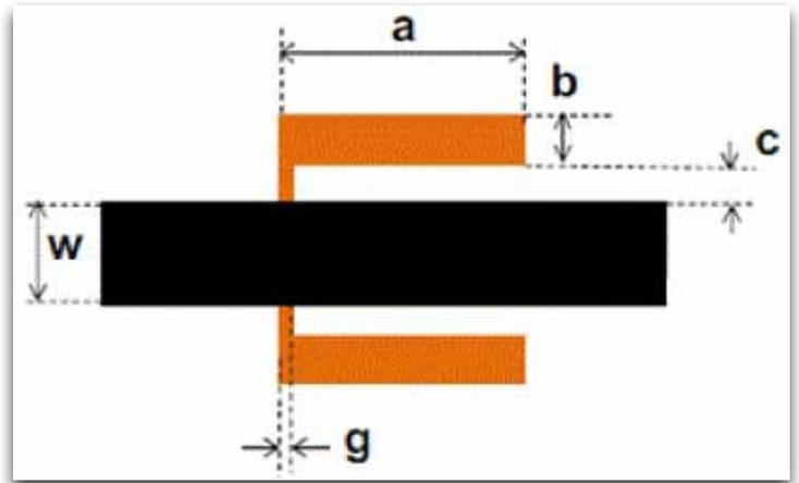
Figure 6: The structure of designed defected ground
