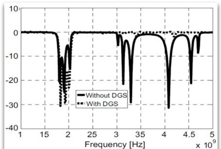
Figure 7: Compare S11 response of proposed filter with DGS plate and non-DGS plate
