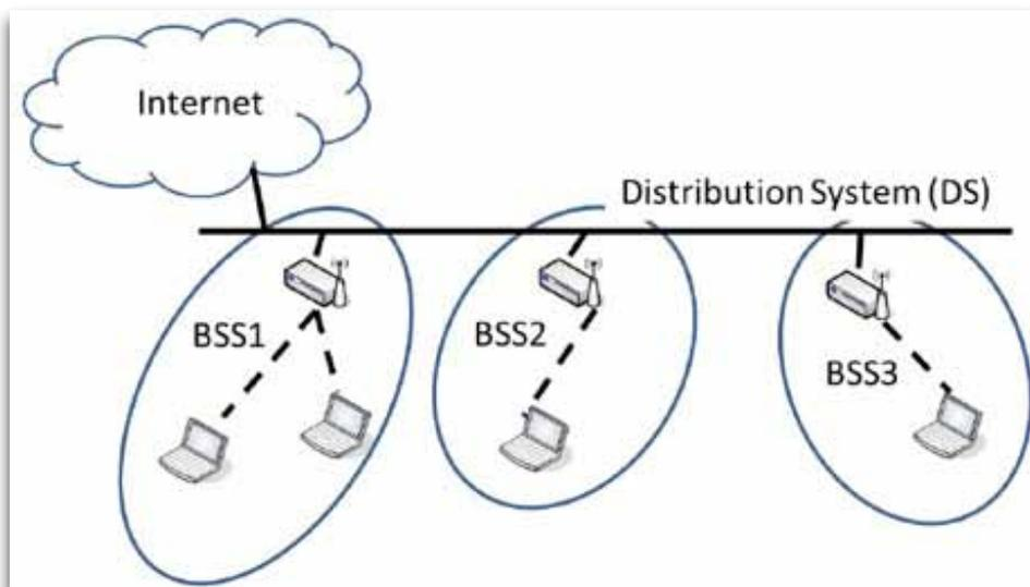
Figure 3: Topology of an IEEE 802.11 Wireless Local Area Network
