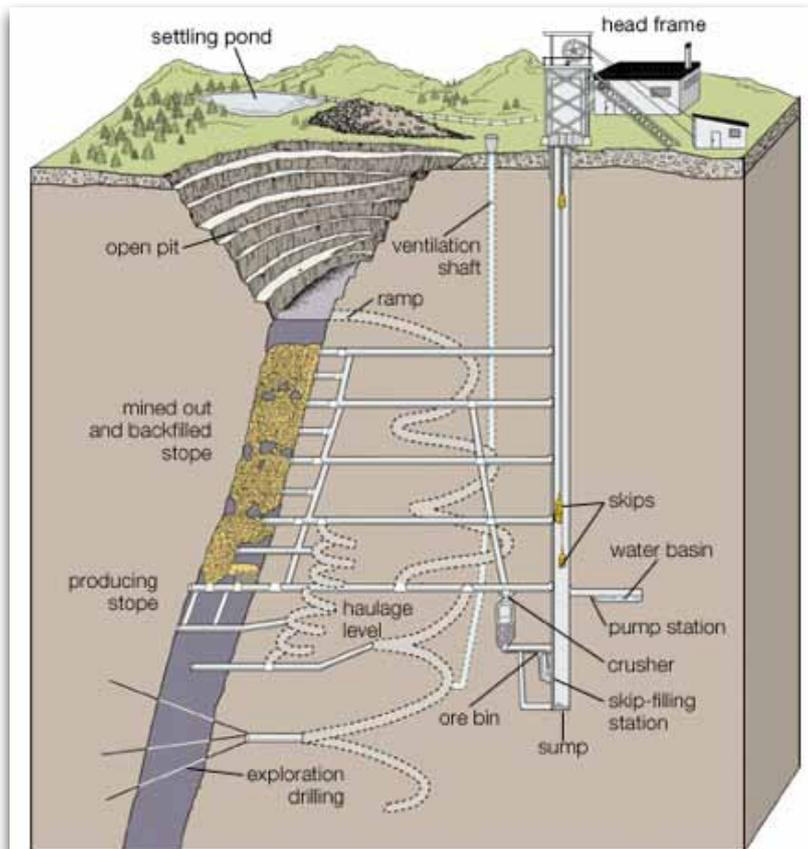
Figure 1: Cross-sectional view of underground mining operations
