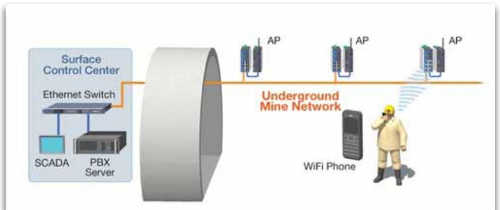
Figure 9: Example of VoIP communications using a Wi-Fi phone [source: 9]
