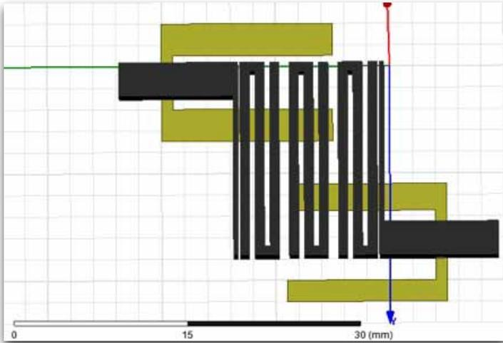
Figure 4: Three-polar band-pass filter with two defected ground units
