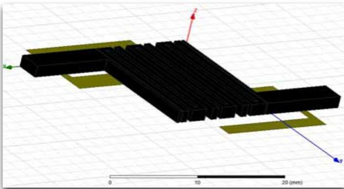
Figure 5: Three-dimensional band-pass filter structure with DGS structure
