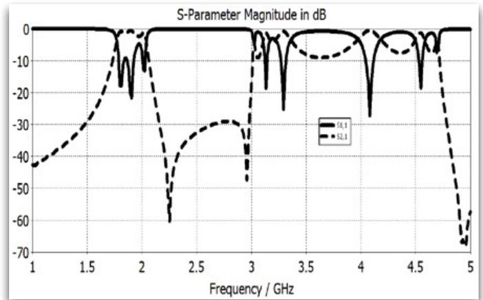
Figure 3: Output of three-polar band-pass filter
