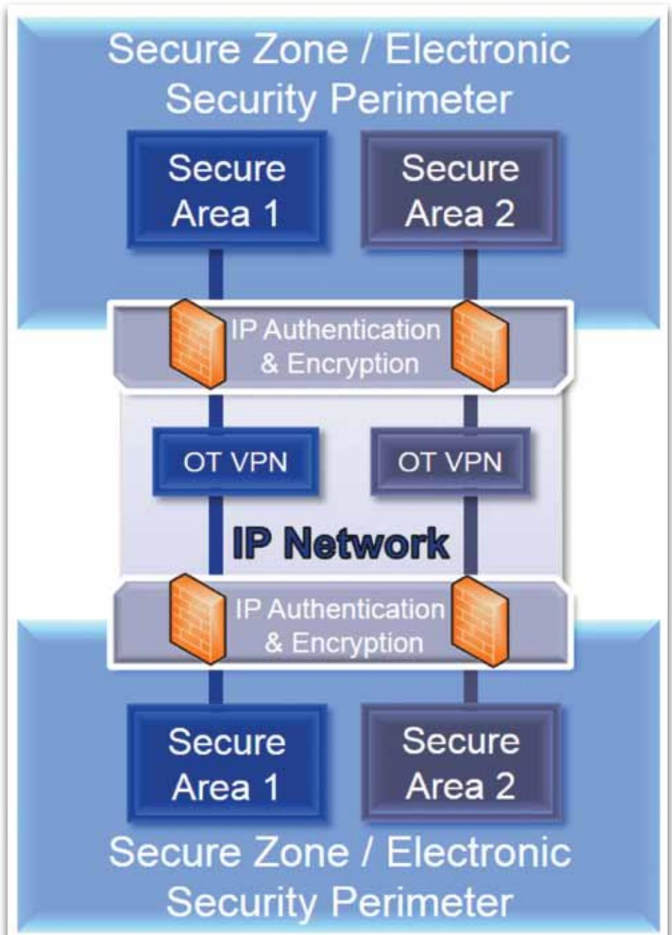
Figure 1: Example secure areas with regards to Secure Zones and Electron Security Perimeters.
