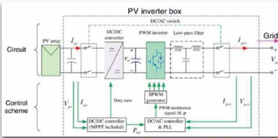
Figure 3: General components arrangement for a typical grid connected inverter [6].
