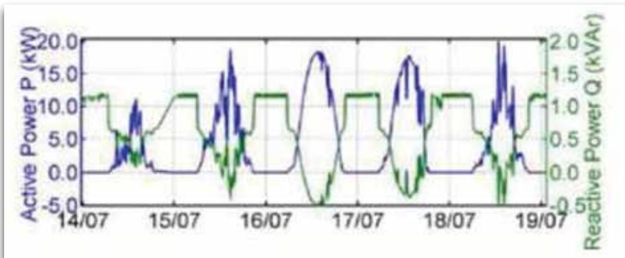
Figure 2: Real and reactive power flow measurements from a unity rated grid-tied inverter [3].
