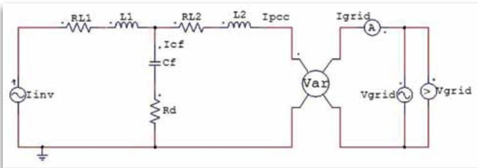
Figure 4: Equivalent circuit diagram for analysis of a grid tied inverter with LCL filter.
