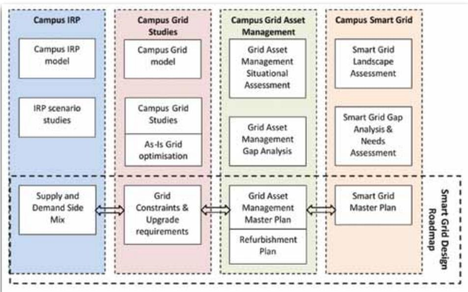
Figure 8: Projects required to develop a Smart Grid Roadmap for te CSIR Pretoria Campus.
