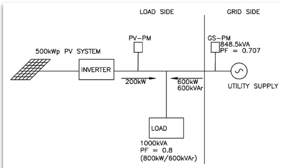
Figure 1: Active and reactive power flow for a load with unity rated power factor grid-tied photovoltaic system.
