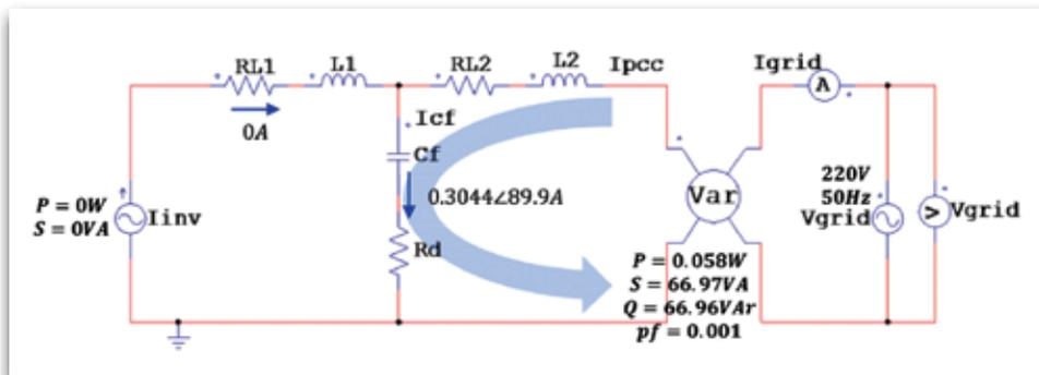
Figure 5: Calculated reactive power and currents caused by the inverter filter when the pv system is producing zero amps.
