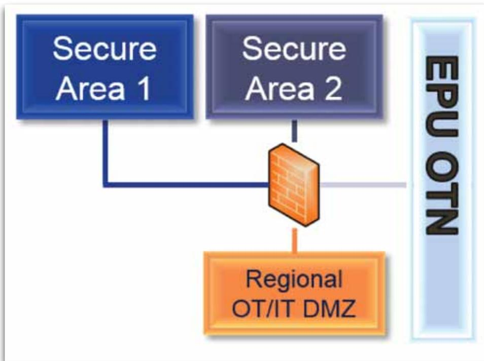
Figure 2: Logical Connection of the OT Secure Areas
