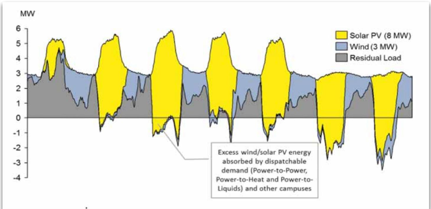
Figure 7: Illustration of campus energy supply with a combination of renewable energy sources.
