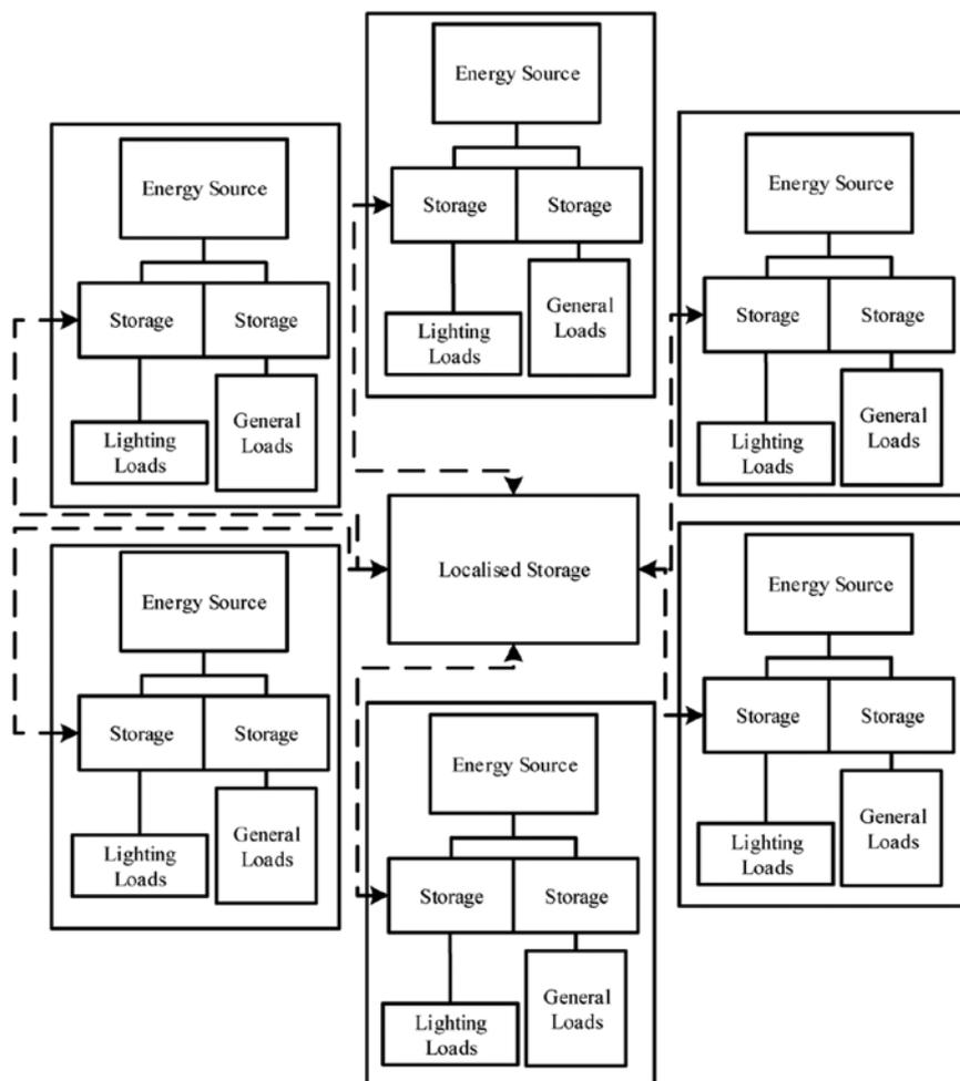
Figure 2: Microgrid Configuration
