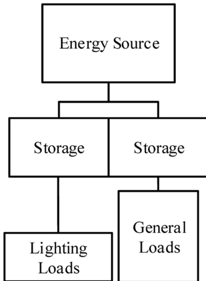
Figure 1: Nanogrid Configuration
