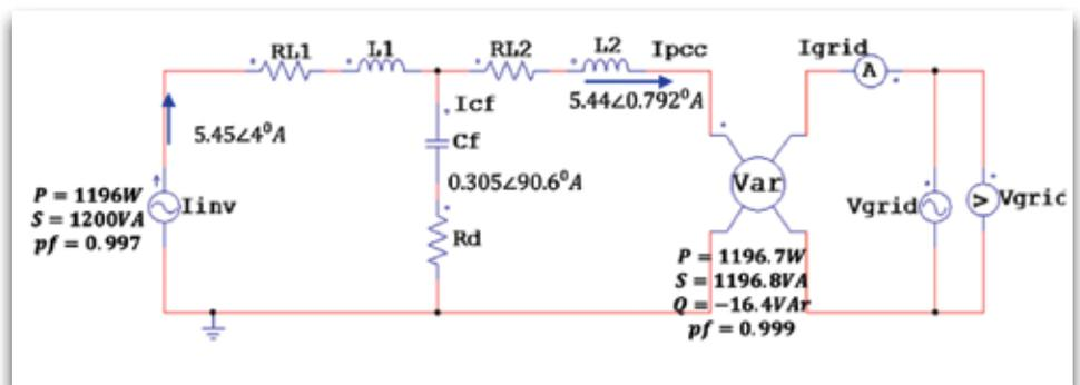
Figure 7: Calculated reactive power and currents caused by the inverter filter, when the pv system is producing 1200 VA at 0.997 p.u. power factor.
