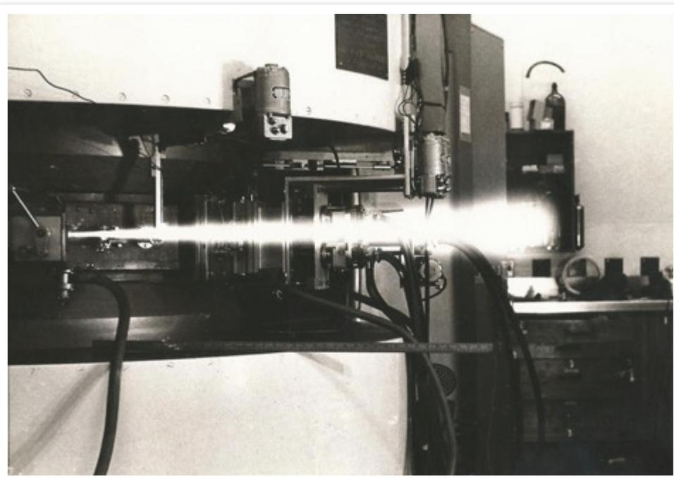
*First external unfocused 16 MeV deuteron beam emerging from the cyclotron.*
