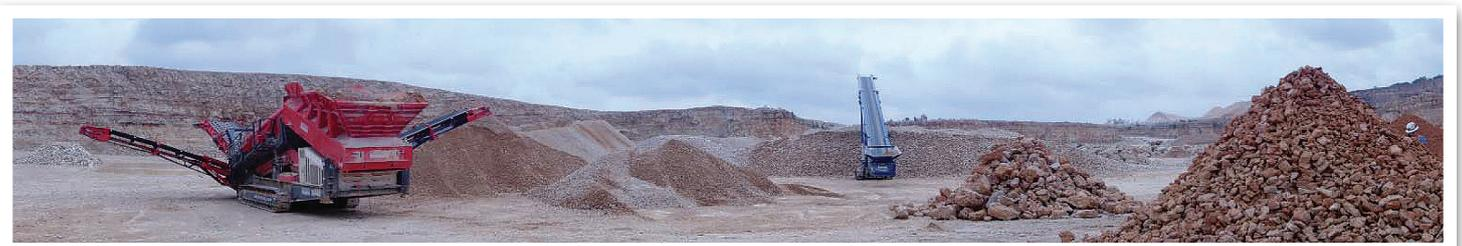
Figure 5. Mobile scalping screen used to sort material.
