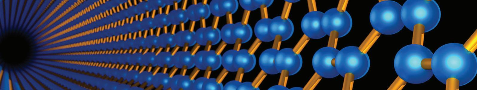
process is active with salinities which exceed that of seawater. The nanotube used for this technique has a diameter of precisely 0,8 nm, a size that causes water molecules to pass single file through the nanotube.
