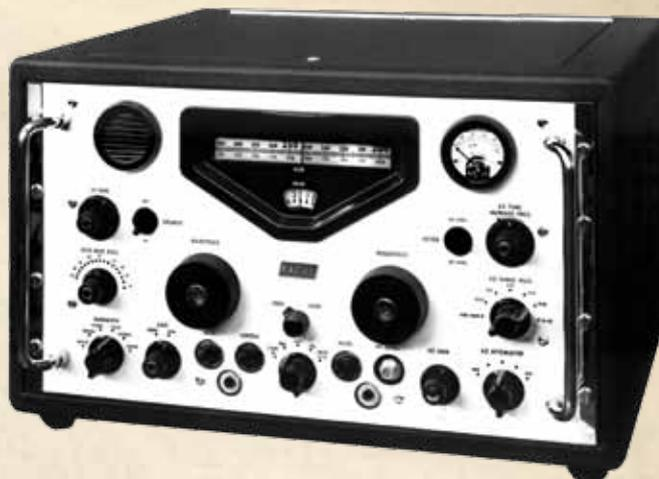
The widely-used 12RA-radio designed by Trevor Wadley.
