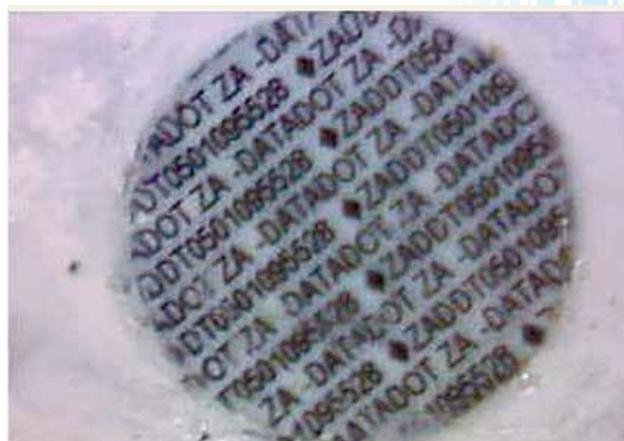
This clearly readable DataDot microdot was taken off the exploded Nissan Almera in a test to prove the permanence of the microdot marking process.
