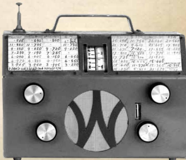
The prototype of the Barlows Wadley radio with a handwritten frequency guide
