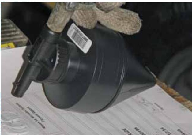
The canister of dots is attached onto a compressed air line and a sample is sprayed onto the fitment sheet.
