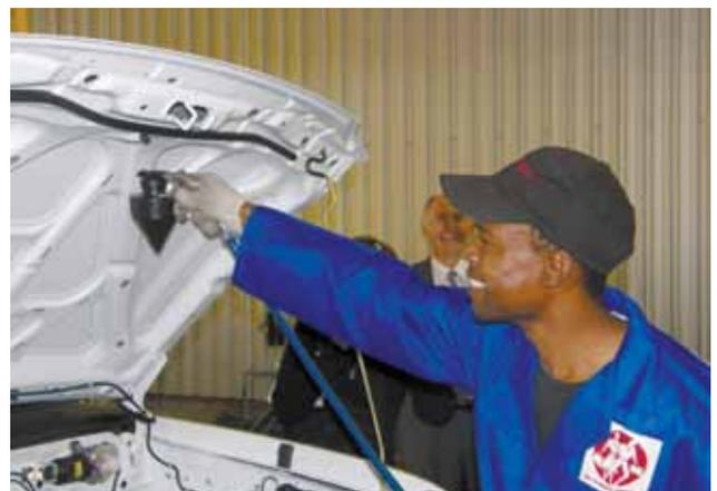
James Ralekwa applies microdots to the engine compartment of a Nissan bakkie.
