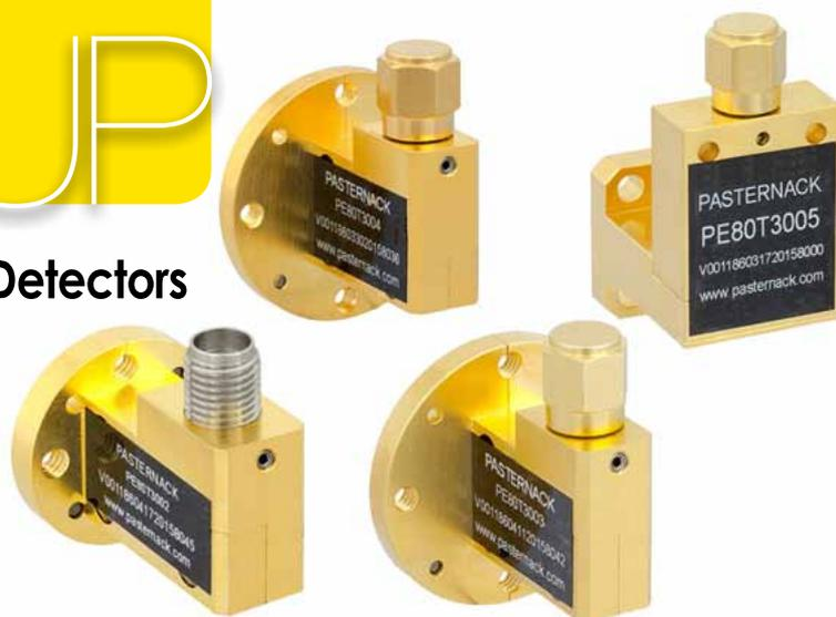
*“This selection of waveguide detectors utilize high performance GaAs Schottky Barrier Beam lead diodes that exhibit high sensitivity performance in Ka, Q, U, V, E and W bands without external DC bias or mechanical tuning,”* explains Tim Galla, Active Components Product Manager at Pasternack. *“Designers will find them particularly useful for applications which involve instrumentation, power detection, power monitoring and direct detection receiver applications.”*
