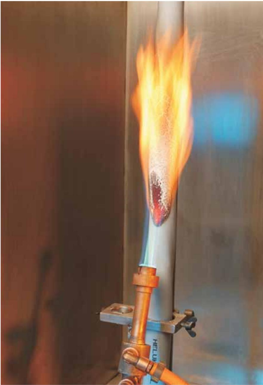
*Helukabel fire testing of cables*
