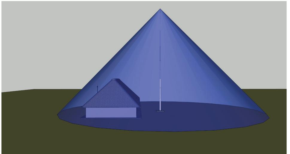
In order to provide the correct lightning protection zones over the entire thatch roof, free-standing masts must be very tall, ranging between 15m and 30m in height.
