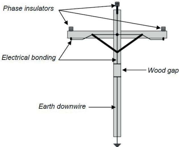
Figure 1 : 300 kV lightning insulation level illustrated on one structure configuration (wood pole and cross-arm used)
