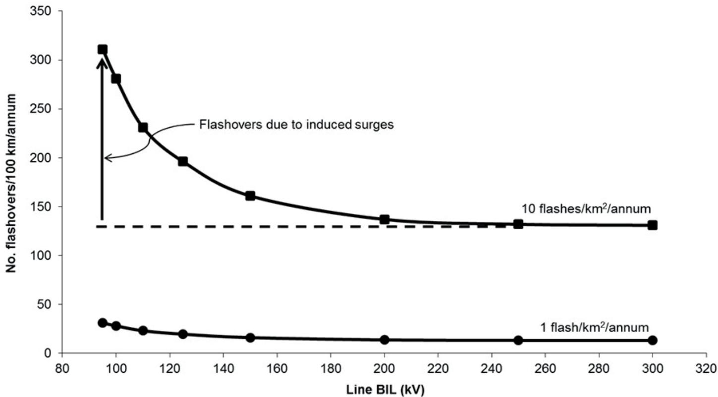
Figure 3 : Number of flashovers due to lightning as a function of BIL (derived from [3] and [4])
