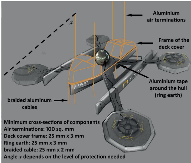
respect to the cost constraints), use of steel reinforcement bars of at least 10 mm diameter could be used to implement the ring conductor. In considering the clearance of the catenary wire and the poles from the protected structure, the sagging and natural inclinations should be considered. The computational method has been described in IEC 62305-3 (2010) [2]. It is recommended to specify approximate values for the clearance distance for a typical housing structure, as a rule of thumb.
