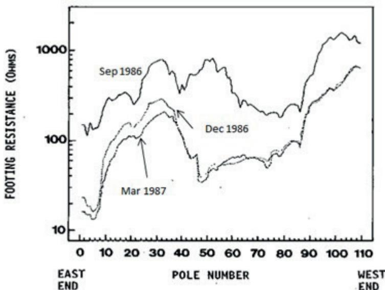
Figure 4 : Test line pole footing resistance (reproduced from [7])
