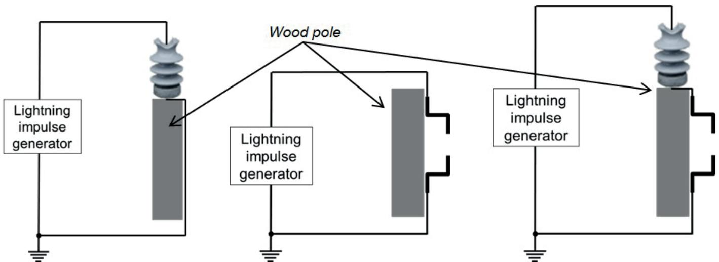
Figure 5 : Lightning impulse laboratory test setup – insulator only (left), spark gap only (centre), insulator and spark gap (right)
