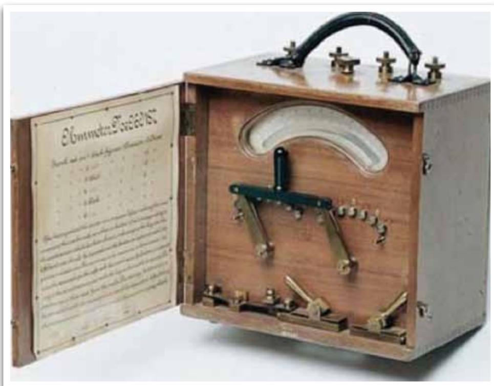
*Portable multi-range laboratory Ohmmeter in wooden case with carrying handle believed to have been used in 1900. It measured resistance up to 1250 ohms.*
