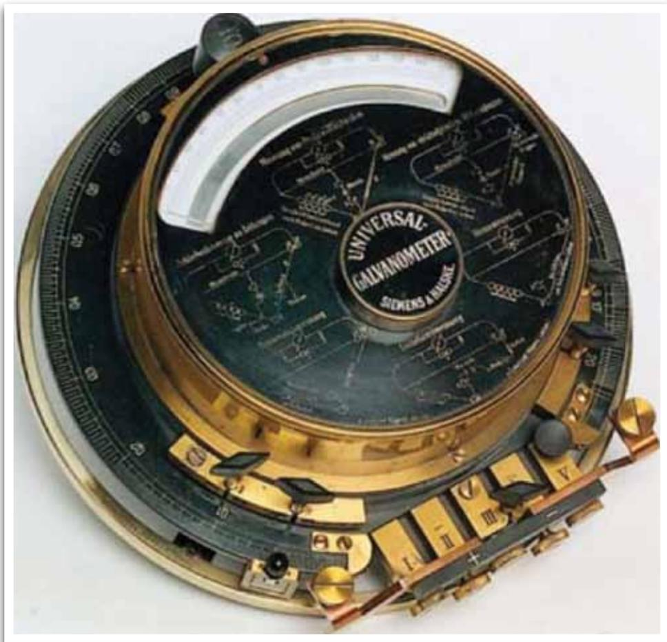
*A Universal Galvanometer made by Siemens and Halske, Germany in 1897. Siemens and Halske supplied this instrument to the Rand Central Electric Works (RCEW) after the construction of Brakpan Power Station in 1897.*
