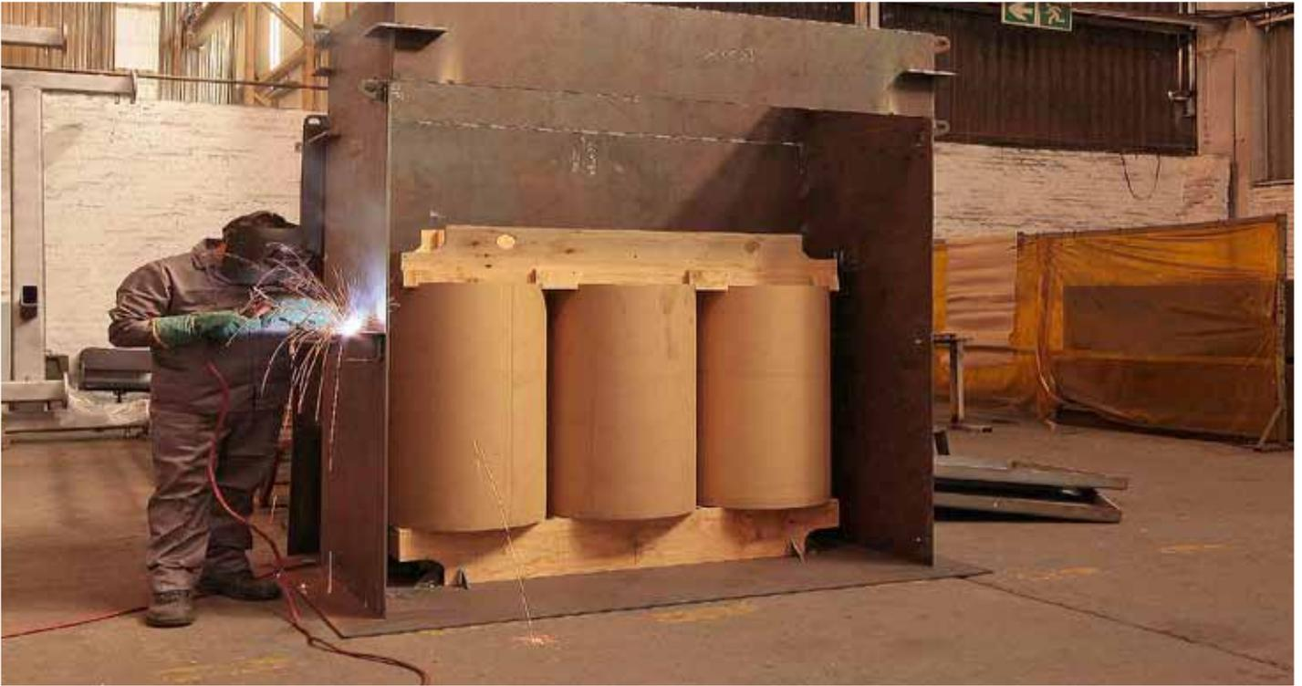
*A welder works on a full-scale model that was made to facilitate achieving the optimum design for the new wind farm transformers.*
