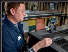
The FLIR DM90 includes Type K Thermocouple input for temperature measurements
