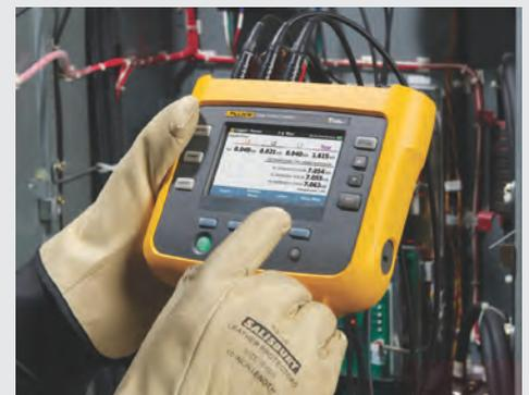
electrical energy waste. These new loggers are easy to set up and use, and capture key measurements - voltage, current, power, power factor, and other variables like temperature - to enable managers to understand their energy usage and correlate it to their activities.
