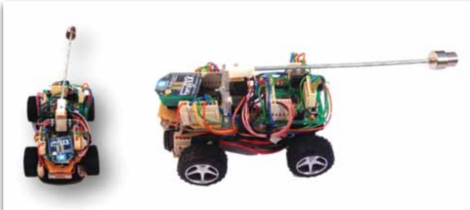
Fig. 2. The TAYObot – the tail actuated stunt robot
