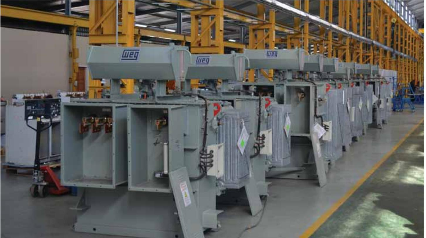
5 x 1 600 kVA 11 kV/433 V and 1 x 2 000 kVA 11 kV/720 V Transformers Export to Ghana
