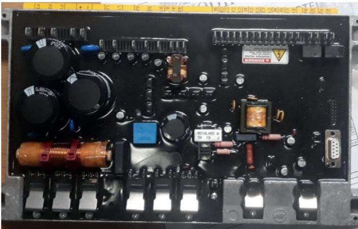
Fig. 5: Automatic Voltage Regulator
