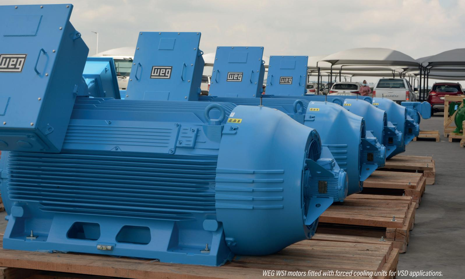
*WEG W51 motors fitted with forced cooling units for VSD applications.*
