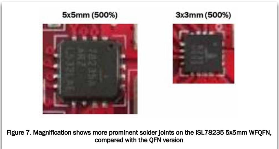
Figure 7. Magnification shows more prominent solder joints on the ISL78235 5x5mm WFQFN, compared with the QFN version
