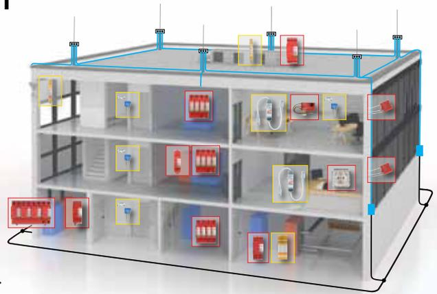
DEHNpatch cables are used to protect terminal devices, whilst the DEHN equipotential bonding enclosure, which can be fitted with LSA disconnection blocks and lightning current carrying DEHNrapid LSA plug-in SPD blocks, can be provided for information technology lines extending beyond the building.
