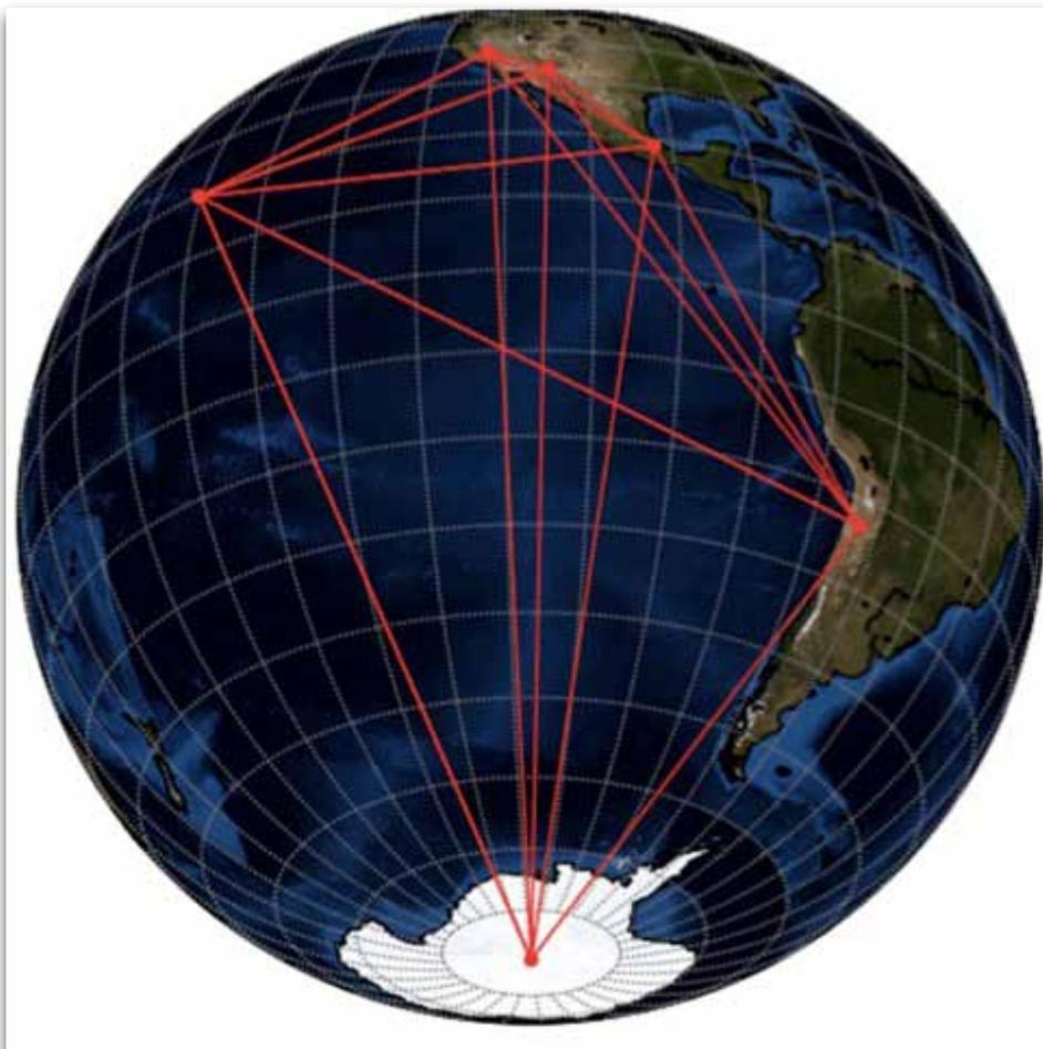
Currently used interferometer baselines with six radio telescopes
