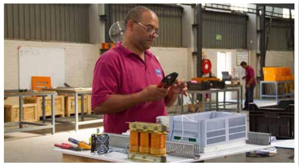
*Assembly of a variable frequency drive panel (VFD) under at Zest WEG Group's facility in Cape Town.*
