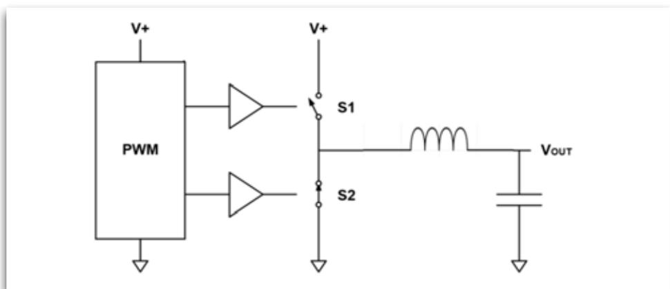
Figure 3. Synchronous buck implementation
