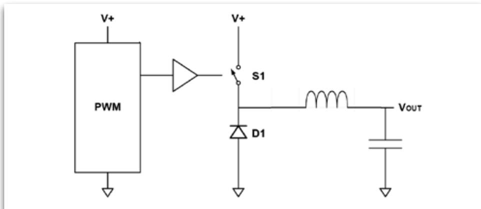
Figure 2. Asynchronous buck implementation
