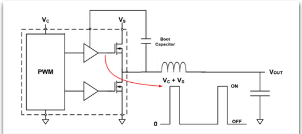
Figure 4. Synchronous buck with N-channel high-side FET switch
