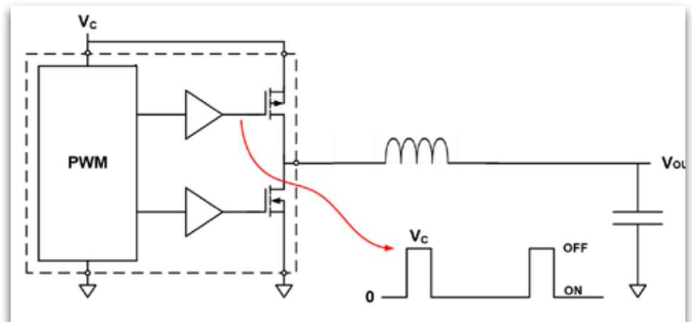
Figure 5. Synchronous buck with P-channel high-side FET switch
