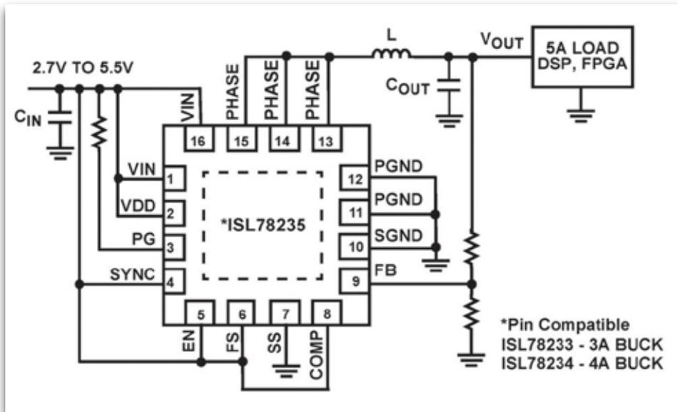
Figure 6. Typical application for ISL78235 5A sync buck regulator
