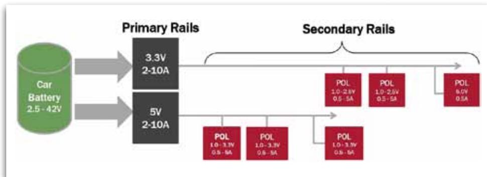
Figure 1. Typical automotive power supply architecture
