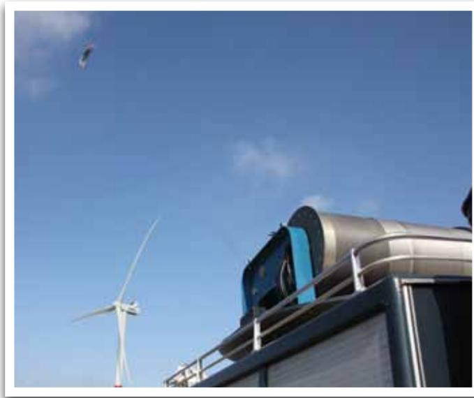
*Figure 4: Size comparison: the kite flies considerably higher than the blades of the windmills and is thereby able to use the higher wind speed present there*
