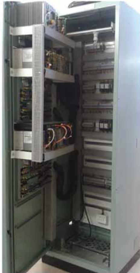
Figure 6: Picture of PMU Scheme -Prototype
