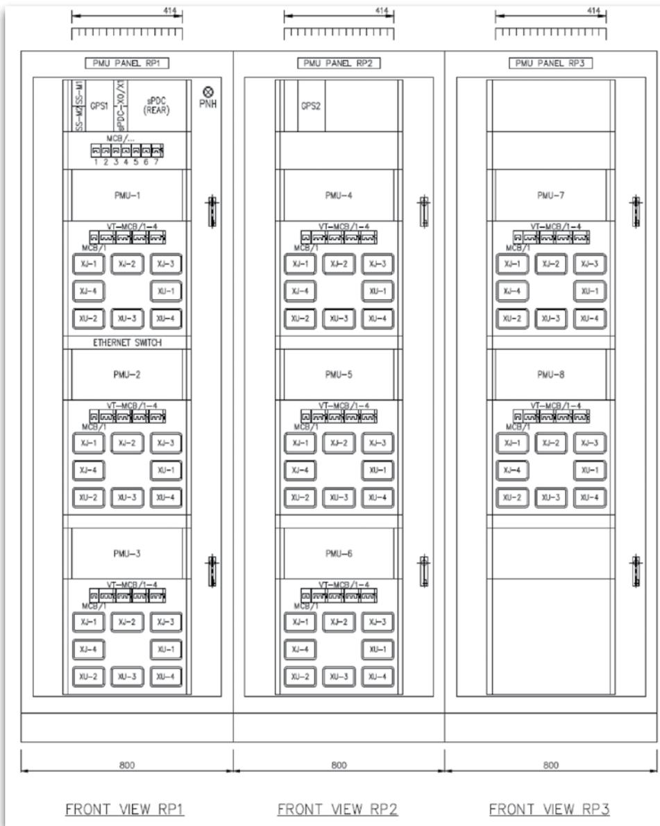
Figure 5: Three panel scheme design incorporating 8 PMUs
