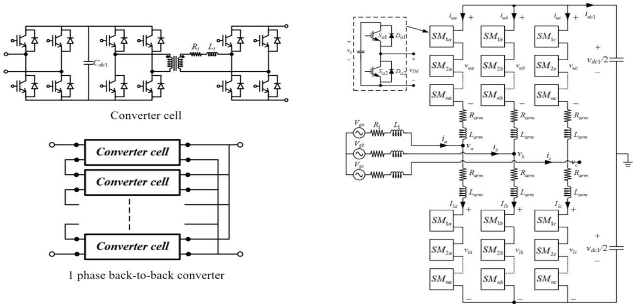
Figure 9: The configuration of a multi-level cascaded SST and configuration for MV based on MMC.
