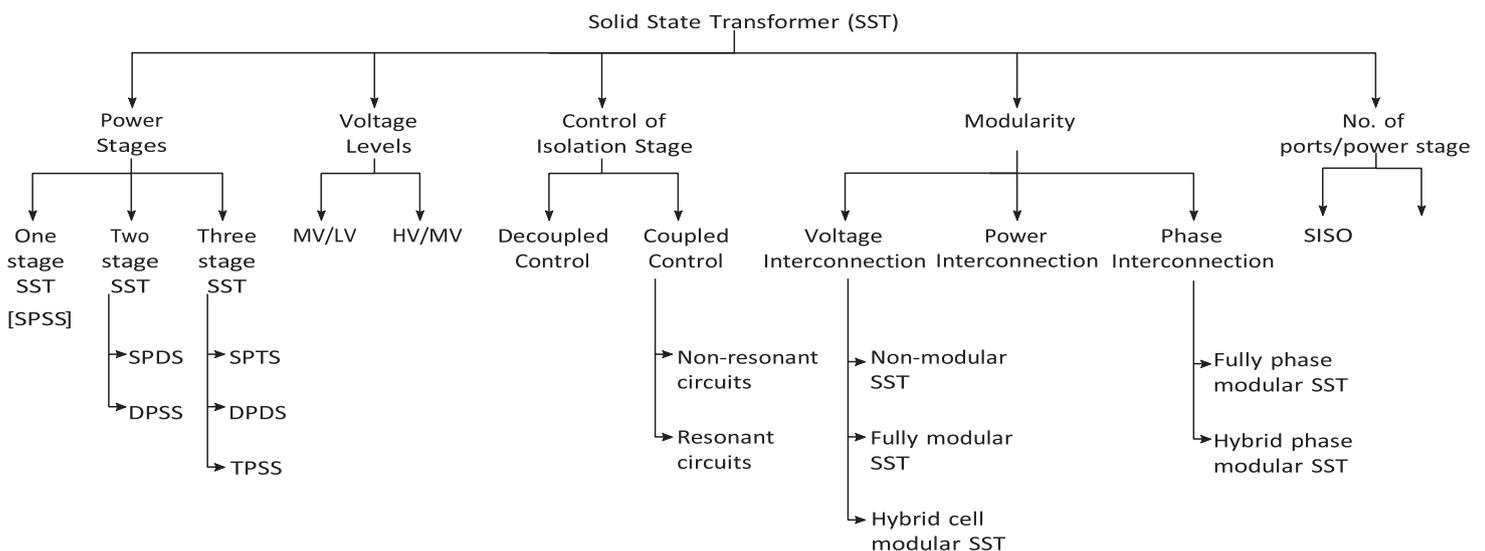
Figure 5: Solid-State Transformer Classifications
