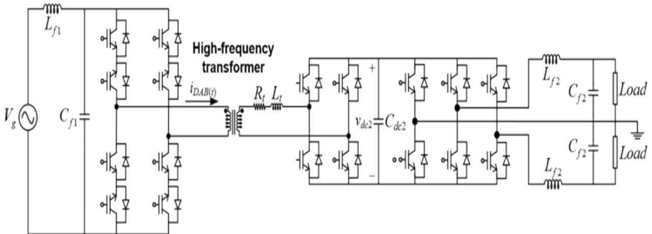
Figure 7: Topology for two-stage solid state transformer.
