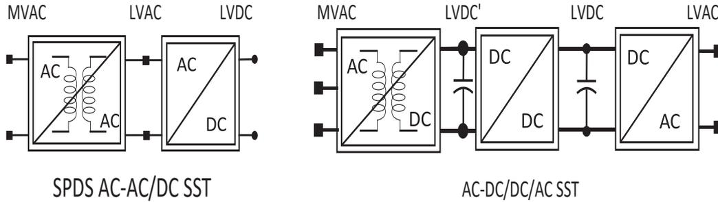
Figure 2: Dual primary single secondary (DPSS) AC/DC-AC SST or single primary dual secondary (SPDS) AC-DC/AC SST.
