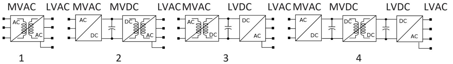
Figure 1: Solid-State Transformer Architectures
