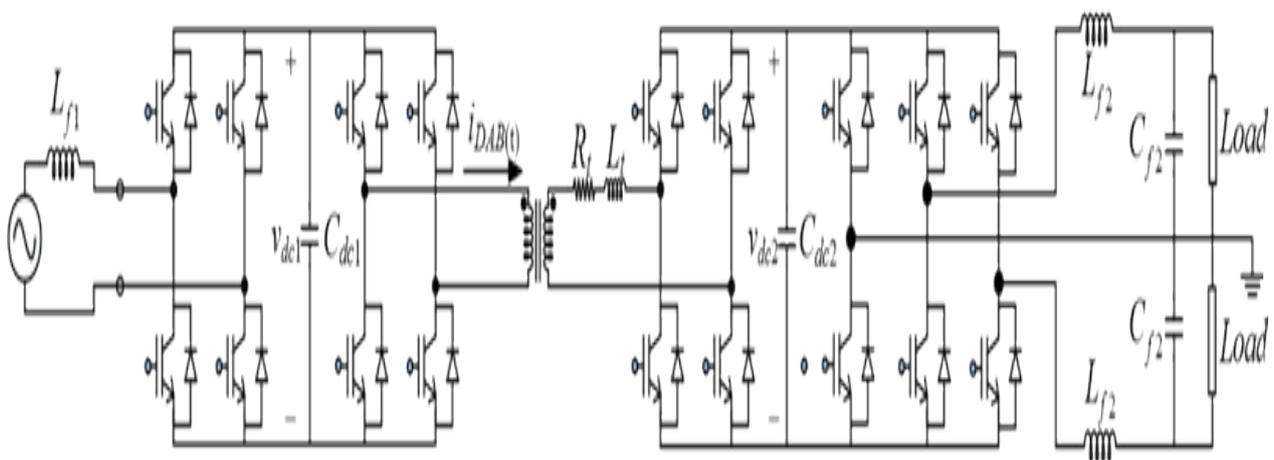
Figure 8: Topology for three-stage solid state transformer.
