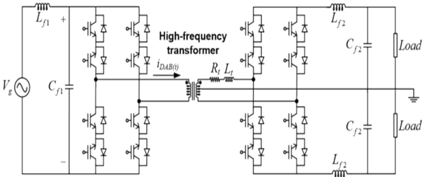
Figure 6: Topology for single-stage solid-state transformer
