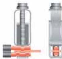
Cables are held in place by spring pressure and deformation on the contact blade.
