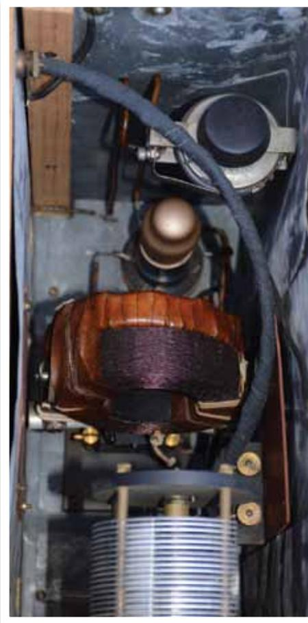
The heterodyne oscillator is constructed in a separate enclosure completely screened with zinc sheeting
