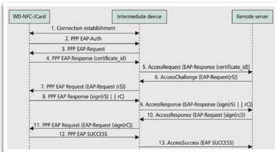
Figure 6 - WD-SCard — authentication server authentication flow
