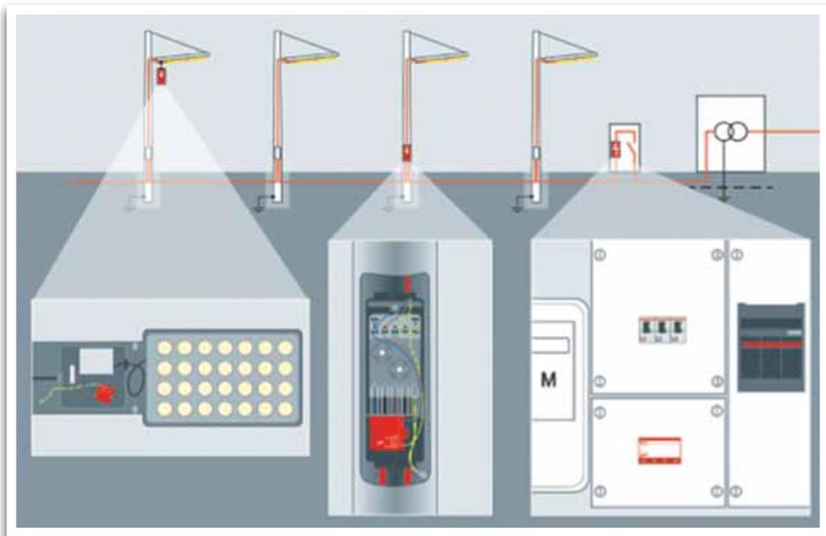
Figure 4: Possible places of installation of surge protective devices in street lighting systems
