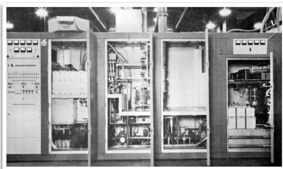
*Fig 2 - Front view of the SSC power amplifier cabinets, showing the interior*
