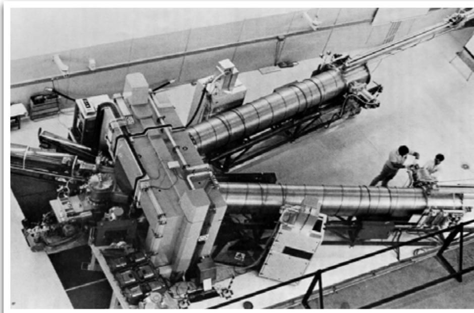
*Fig 1: The solid-pole injector cyclotron with two resonators and their power amplifiers in position.*
