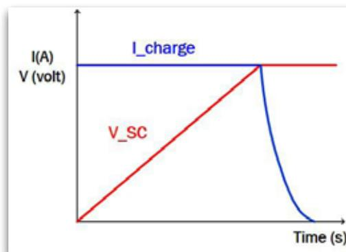
Figure 2. CICV Supercapacitor Charge Control
