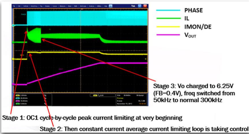
Figure 5. Bench Waveforms of SC Charging
