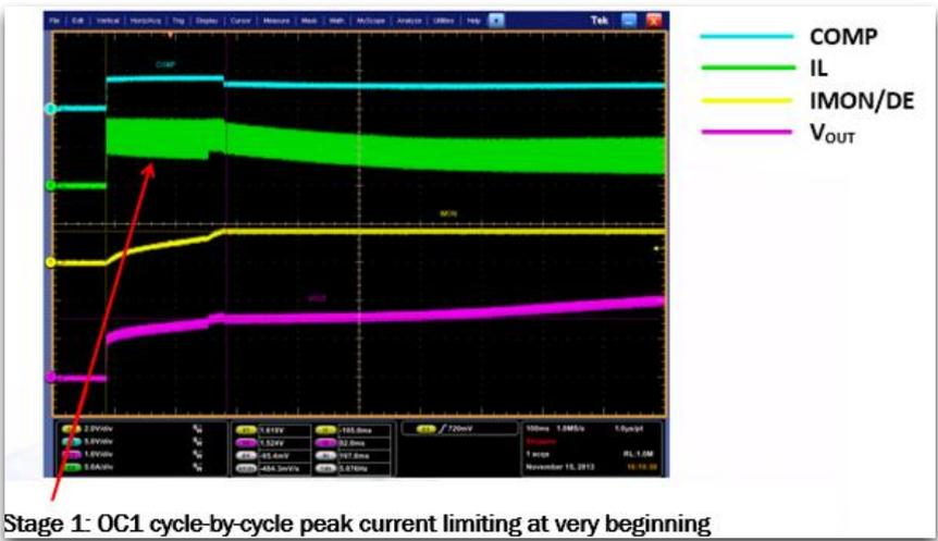
Figure 6. Zoom in Bench Waveforms of SC Charging at Stage 1
