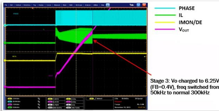
Figure 7. Bench Waveforms of SC Charging
