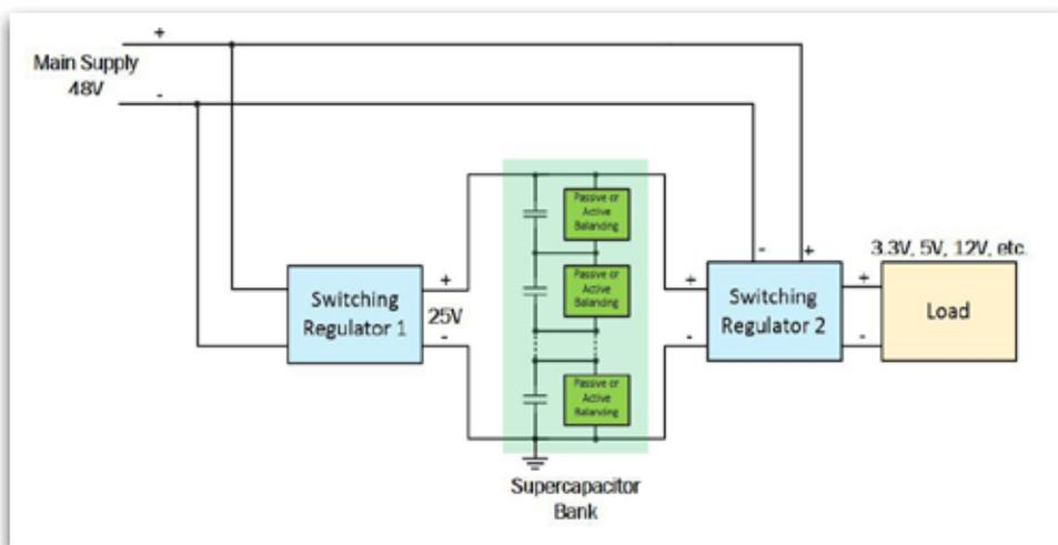
Figure 1. Block Diagram of a Battery Backup System Example using a Supercapacitor Bank
