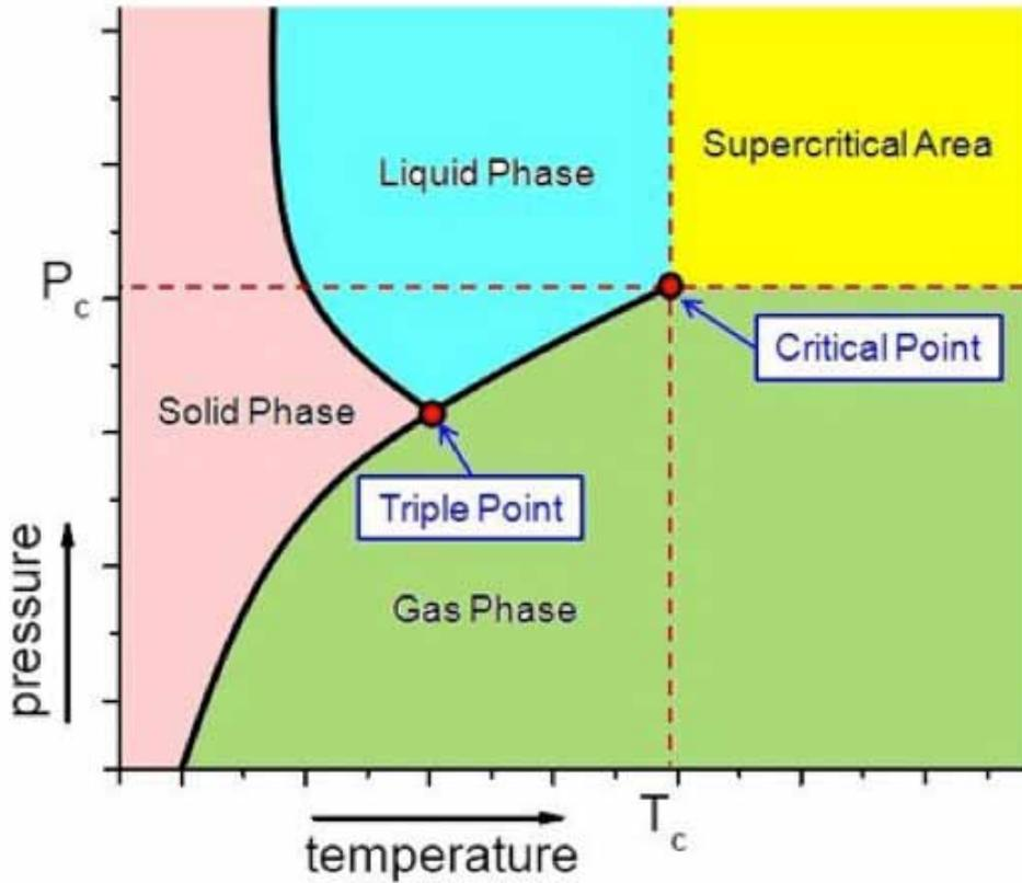
oxygen free water which is continuously circulated. If it is required to improve the power station efficiency even further, it becomes necessary to consider ultra-supercritical water. The furnace, turbine, condenser circuit of the thermodynamic fluid is represented by the Rankine cycle.
