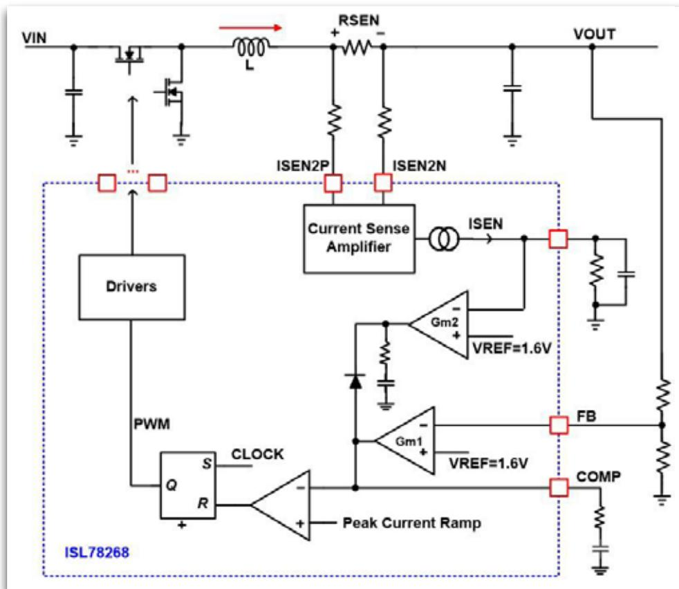
Figure 4. ISL78268 CICV Loop Simplified Block Diagram
