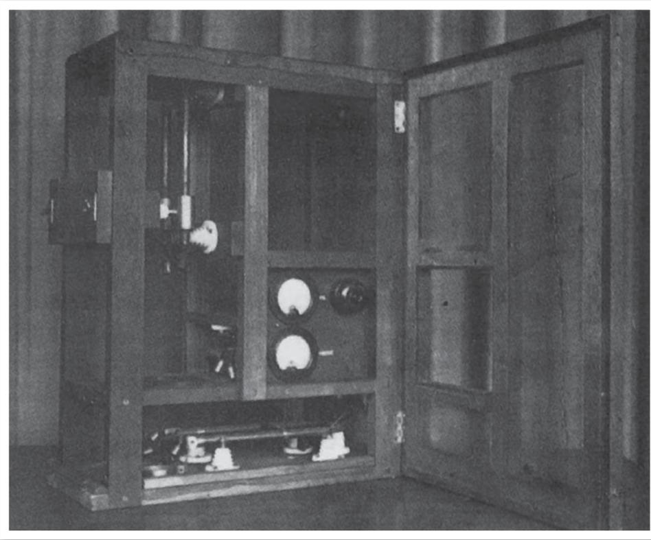
*JB1 radar transmitter without its valves.*
