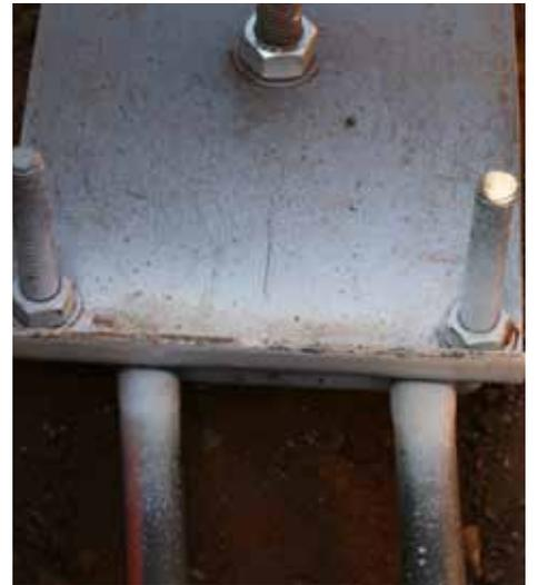
6. This is a close-up of the front plate, closest to the side where the machine exerted the pressure to pull the cable out, but was only able to break the cable. No movement is visible on the paint on the cable, or the device.
