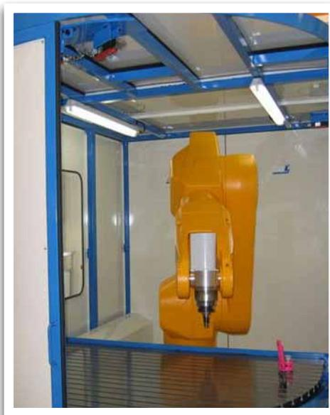
*Milling robot in an enclosed work cell.*
