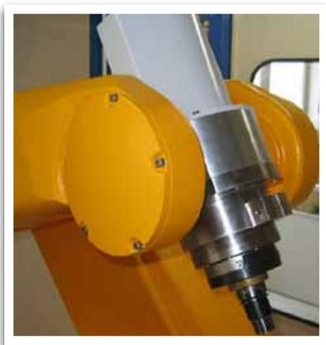
*Detail of a milling robot's tool*
