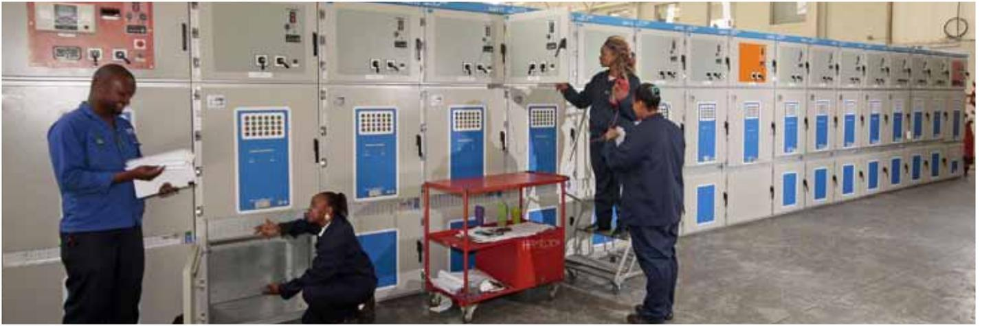
*ACTOM MV Switchgear technicians completing assembly and inspection of the AMV12 switchgear panel for City Power's Industria substation*
