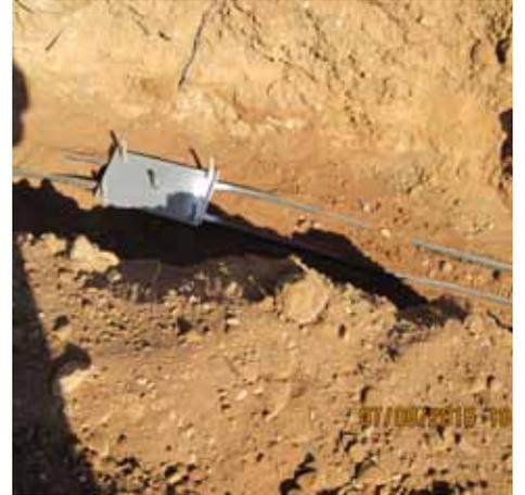
5. A view of the first plate in the trench, after the trench had been opened up after the test had been completed. No movement to the plate, nor to the anchor was evident; even after the anchor had been dug out of the ground, together with the concrete. No damage to the foundation was found either.
