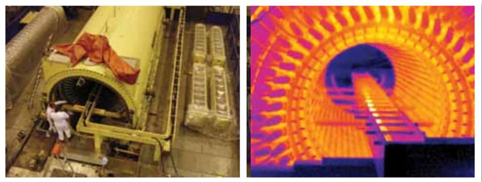
*Fig 6: Rated Flux Test Setup and View Through Thermal Camera on a 600 MW stator*
