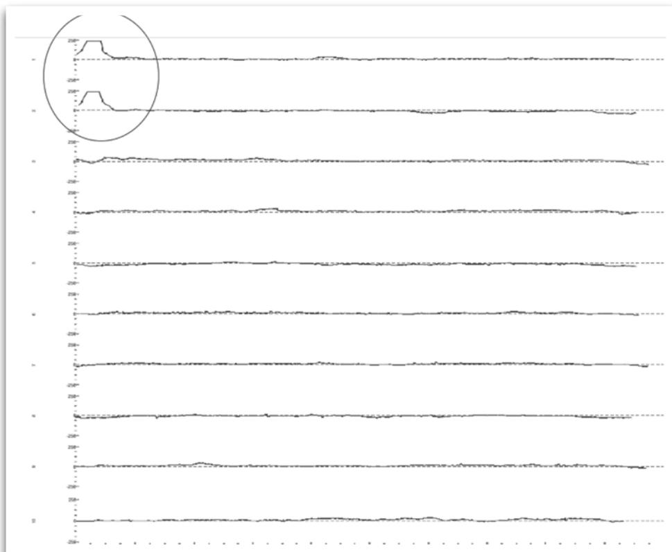
Fig 10: Overview of EL CID Results Showing Fault in Slot 1
