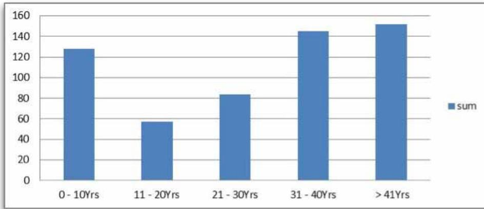
Figure 2: Eskom Transmission transformer age distribution
