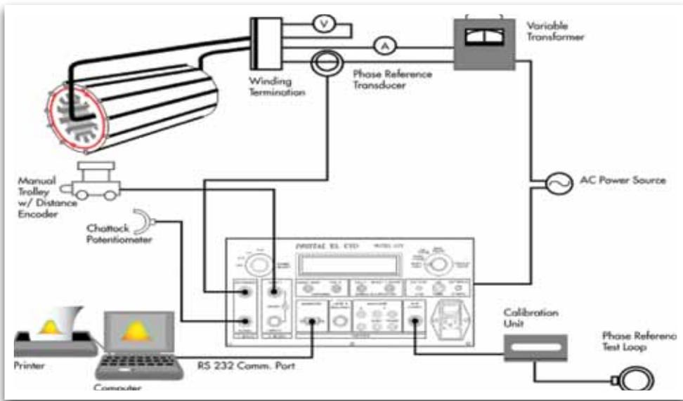
Fig 2: Sketch from EL CID Manual showing EL CID Test Setup
