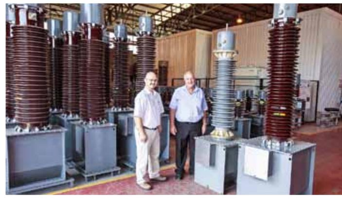
*Nick de Beer (right), Product Manager, Instrument Transformers, and Etienne Venter, Design Engineer, Voltage Transformers, of ACTOM High Voltage Equipment stand next to a compact 132kV voltage transformer, which is substantially smaller than the conventional units around it, as the picture shows.*
