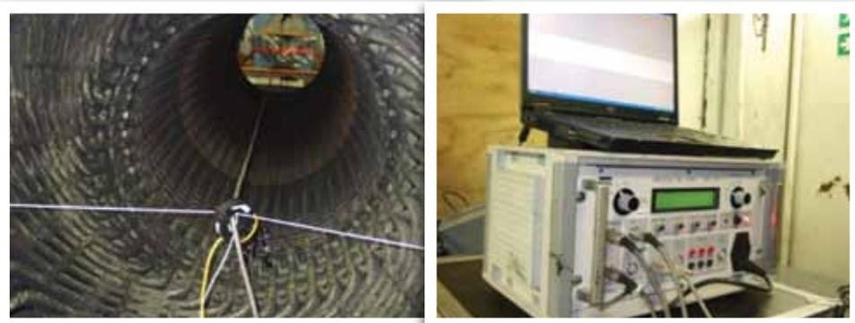
Fig 4: ELCID Test Setup for conventional test
