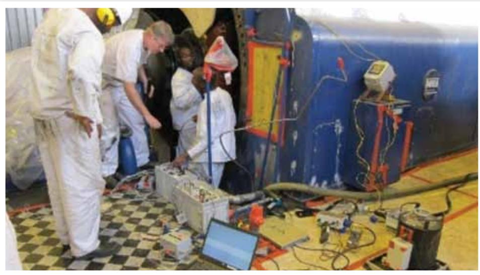
Fig 3: ELCID Test Setup for Rotor In-situ test
