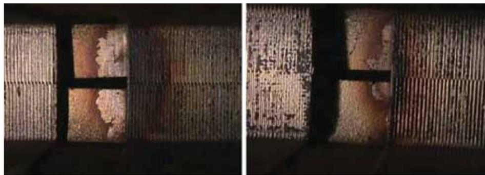
*Fig 23: Close up View of the Hotspots Between the Vent Duct Spacer and the Core Laminations.*
