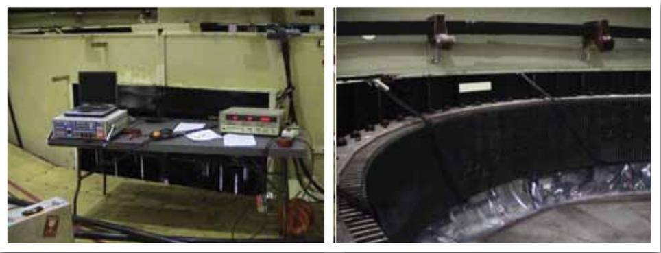
*Fig 5: Rated Flux Test Setup on a Hydro Stator Core*
