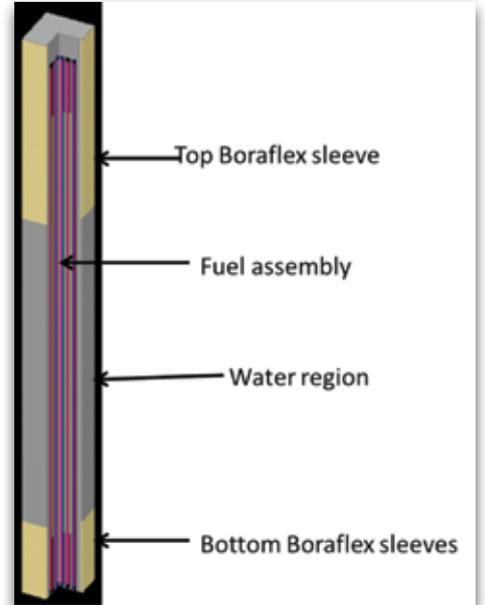
Fig. 5: Boraflex sleeves at the top and bottom end of the fuel assembly
