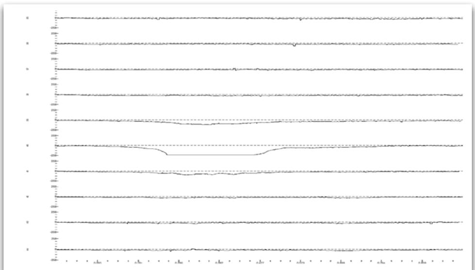
*Fig 7: EL CID Overview Results for slots 35 – 45*
