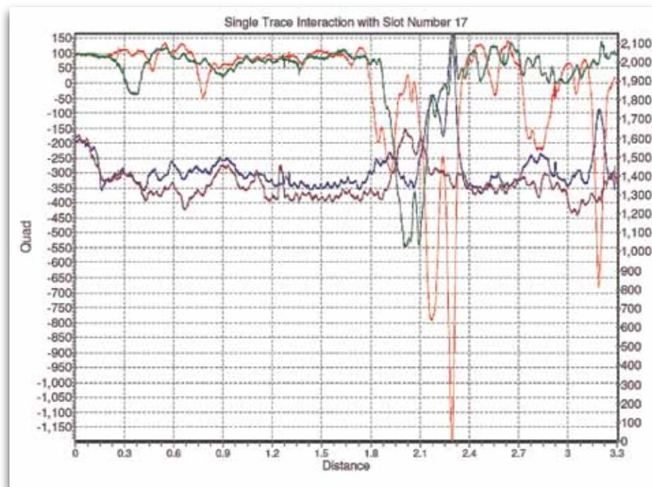
Fig 16: Close up showing the results in slot 17 (Red Trace) overlaid with the results in slot 18 (Green Trace).
