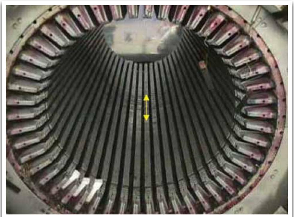
Fig 22: Photo of the Core Showing the Vented Section in the Middle.
