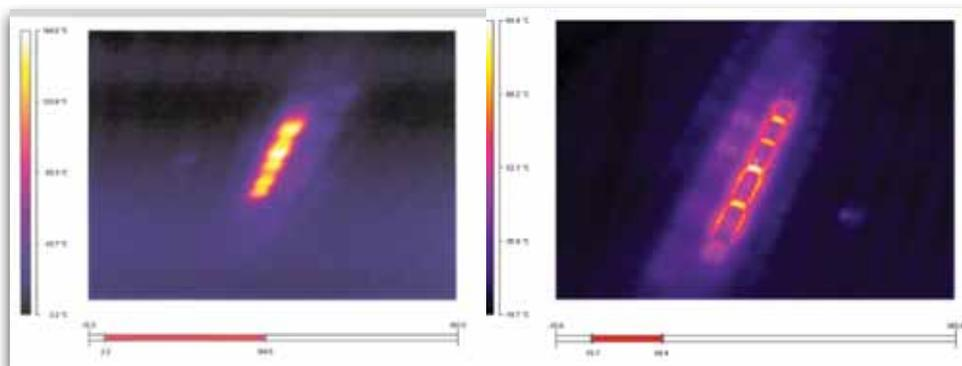
Fig 9: View of slot 40 through Thermal Imaging Camera Before and After a Repair Attempt
