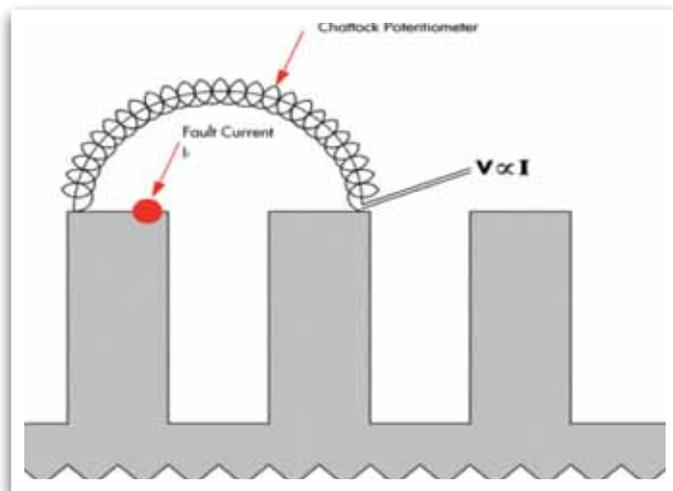
Fig 1: Sketch from EL CID Manual of the Chattock Potentiometer
