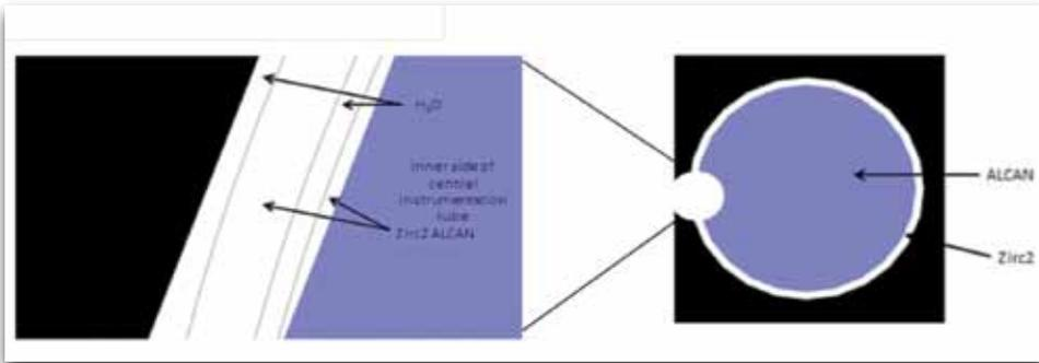
Fig. 7: Neutron absorber insert as a cord in the central instrumentation tube
