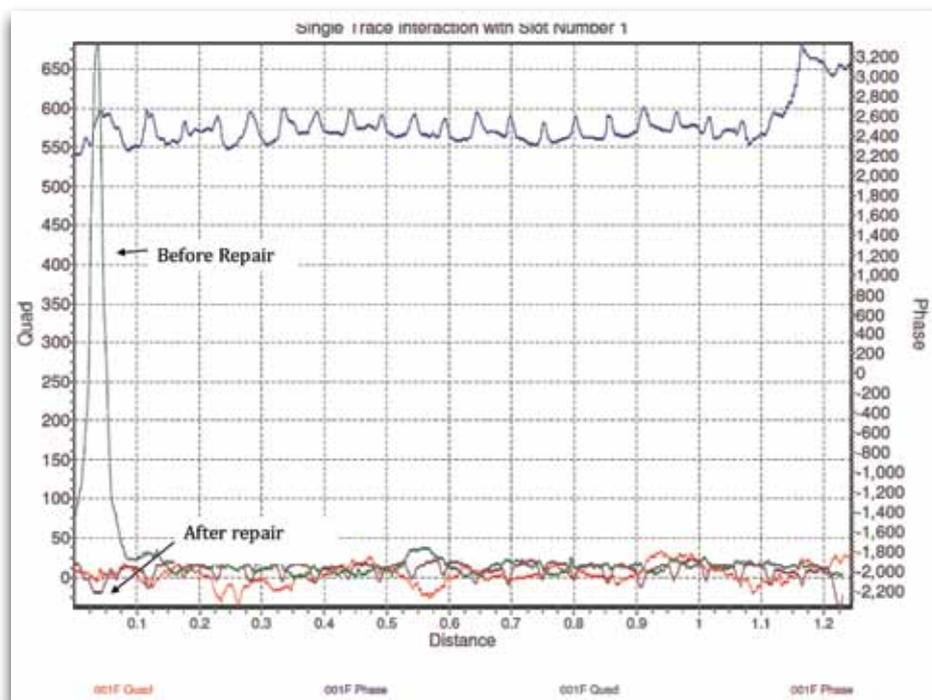
Fig 14: Close Up View Showing the Before Reading in slot 1 (green trace) and After (red trace).
