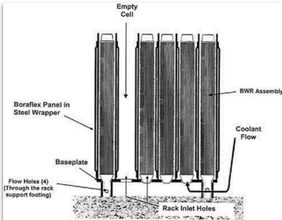
Fig. 1: Boraflex as an absorber insert [9]
