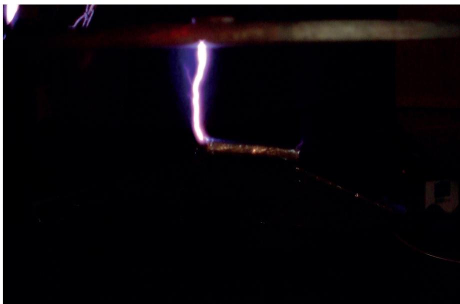
*Figure 7: Representative photograph of gap-bridging positive leader originating from the model (3s camera exposure). The gap bridged by the leader in this configuration was 26cm.*
