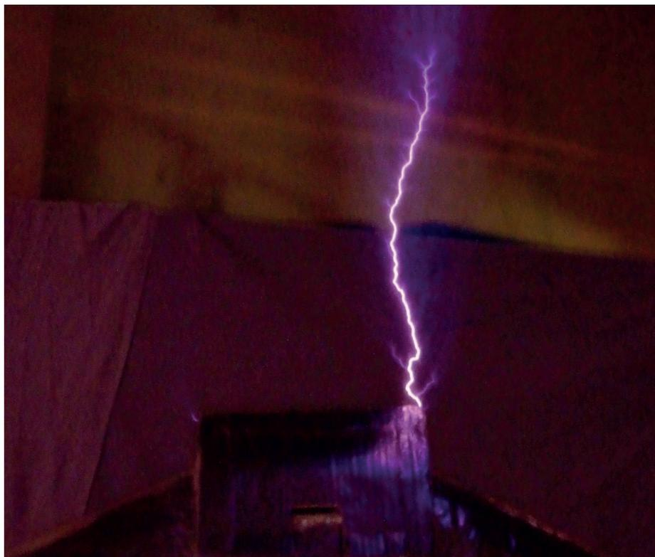
*Figure 6: Representative photograph of aborted positive leader originating from the model (3s camera exposure). The total length of this aborted leader, measured along the leader path and accounting for its tortuosity, is 44cm.*
