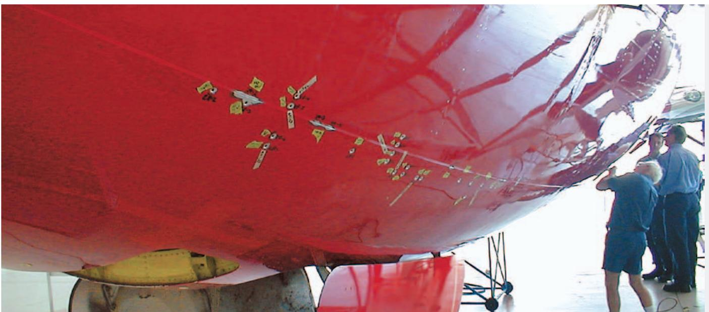
*Figure 6: Damage caused by lightning moving along an aeroplane
