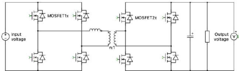
Figure 7. Bidirectional Dual Active Bridge
