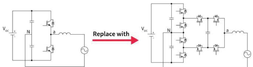
Figure 3 Replacing a two-level topology with a multilevel topology
