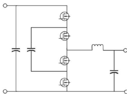
Figure 6. Three-level Bidirectional Flying Capacitor Converter
