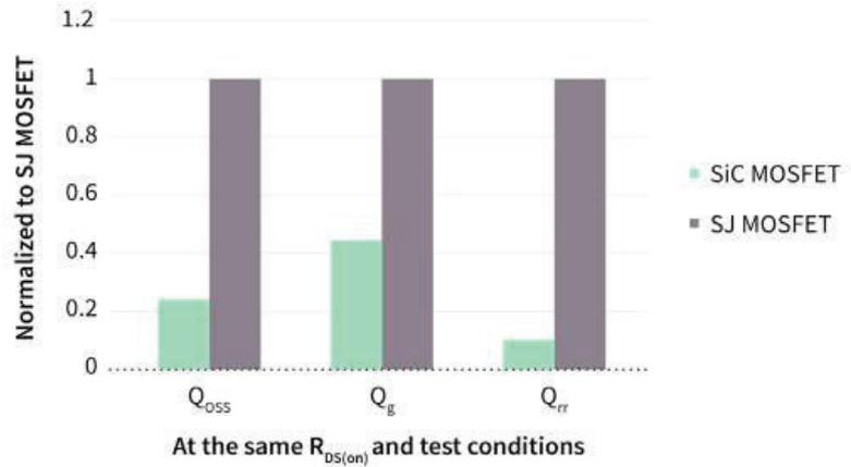
Figure 1 Comparing figures-of-merit for SiC and SJ MOSFETs at the same operating conditions and  $R_{DS(on)}$
