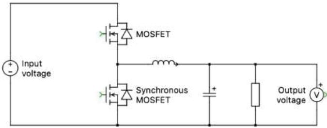
Figure 3. Synchronous Buck
