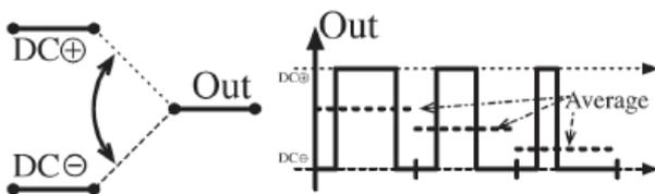
Figure 1: Two-level Topology Operation
