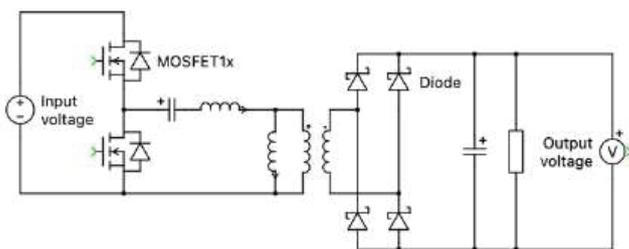
Figure 8. Half-bridge LLC Converter
