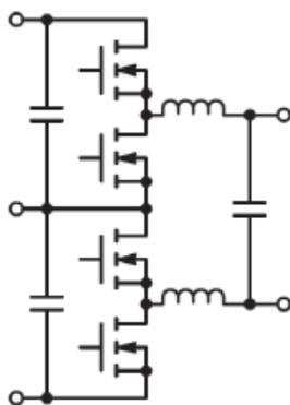
Figure 5. Three-level Symmetric Buck-Boost
