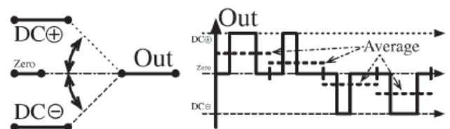
Figure 2: Three-level Topology Operation
