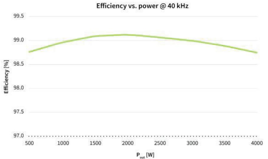
Figure 5 Efficiency vs. output power for the five level inverter (@ 40 kHz switching frequency)
