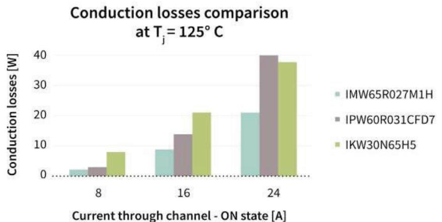
Figure 2 Comparing device conduction losses at 25°C (left) and 125°C (right)
