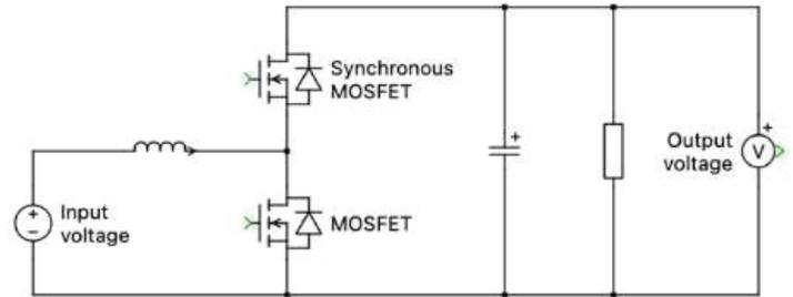
Figure 4. Synchronous Boost
