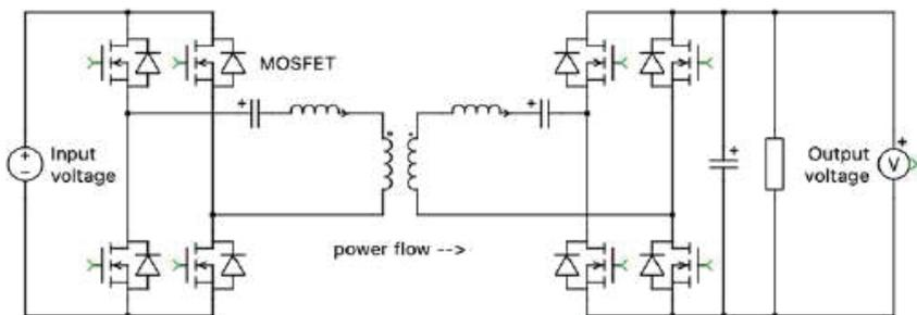
Figure 10. Bidirectional CLLC Converter
