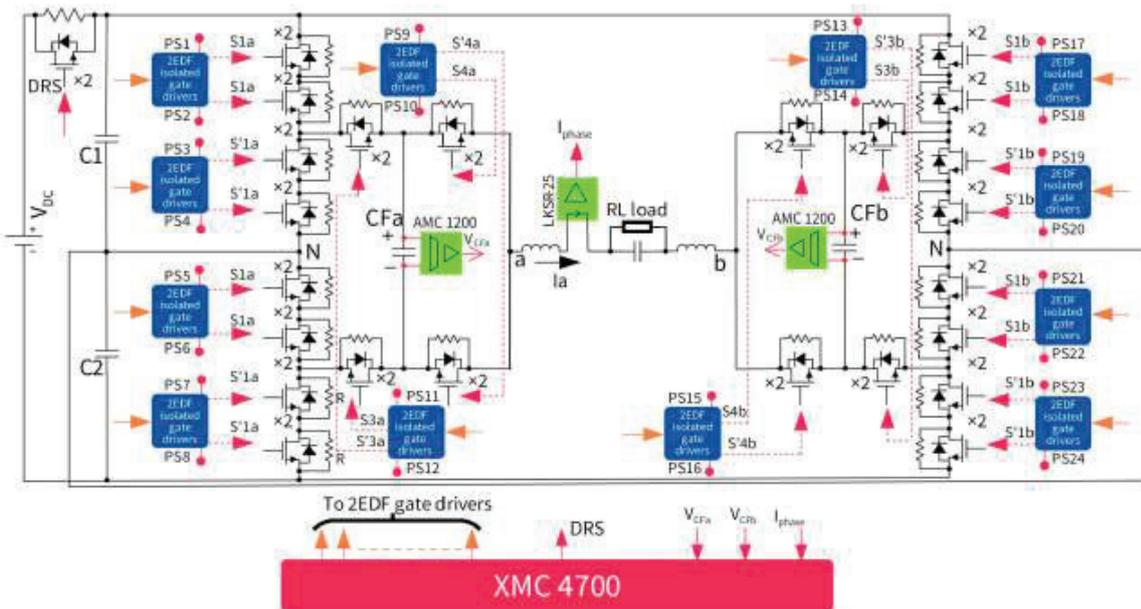
Figure 4 Schematic of the five level inverter design
