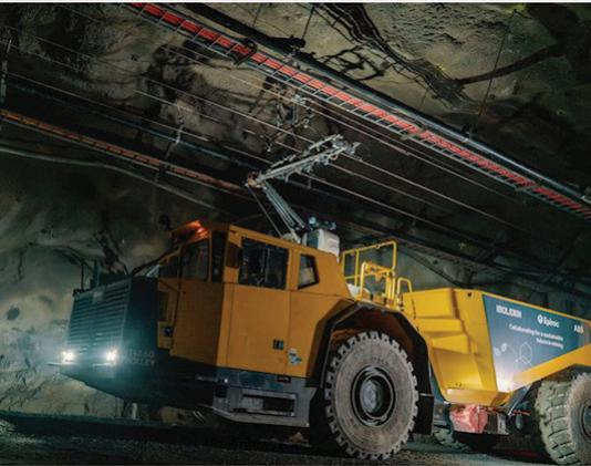
**Boliden, Epiroc, and ABB have passed a new technology milestone by successfully deploying the first fully battery-electric trolley truck system on an 800-meter-long underground mine test track in Sweden, with a 13 percent incline. This means the mining industry is a step closer to realising the all-electric mine of the future, with sustainable, productive operations and improved working conditions.**
