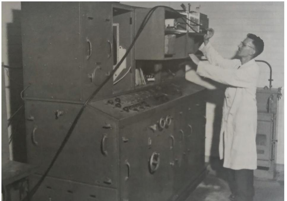
*Figure 3: Jules Fejer adjusting the equipment used at the TRL to measure particle reflections, cross modulation and absorption in the ionosphere.*
