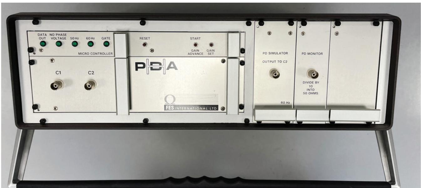
Figure 5: First Commercial Digital Instrument Measuring PD in the 30- to 300-MHz Range
