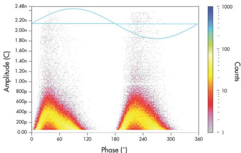
Figure 4: Phase-Resolved PD (PRPD) Plot of PD Magnitude vs. AC Phase Position
