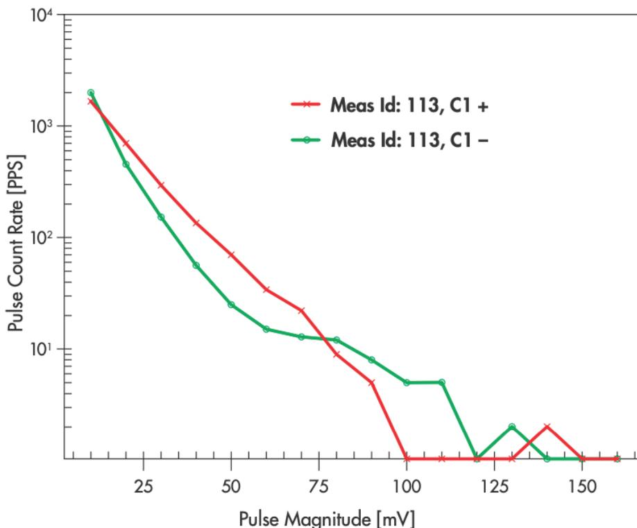
Figure 3: Pulse Magnitude Analysis Plot for Each Polarity of PD Pulses
