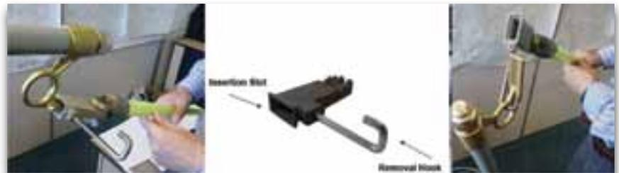
Figure 10: The insertion tool to replace drop out surge arresters & fuses
